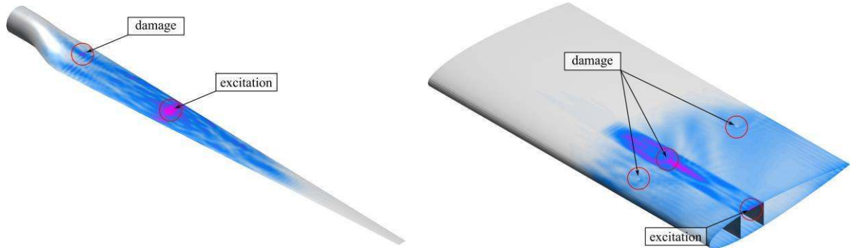
Figure 4: Calculated weighted RMS patterns of propagating guided elastic waves in: a composite wind turbine blade with a crack (left), an aluminium wing section with damage (right), shell structure according to a six-mode theory of shells [16] – results of numerical simulation obtained by TD-SFEM for a 8 sine pulse excitation signal of 75 kHz modulated by the Hann window.
