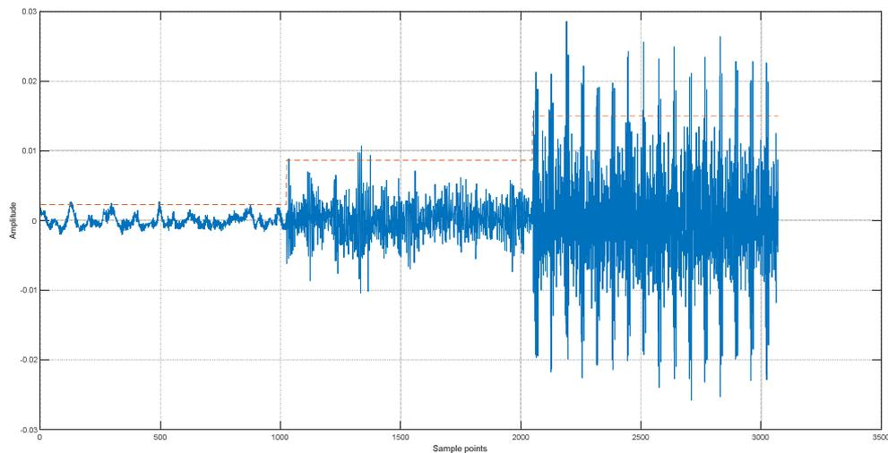
Figure. 4 Signal with improper backlash and the alarm level
