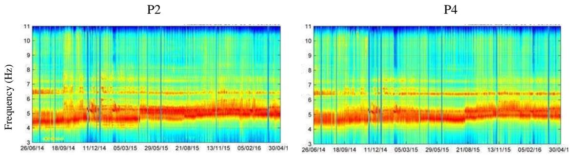
Figure 9: Colour maps with the time evolution of the frequency content of the acceleration time series measured at the top of piers P2 and P4 along the longitudinal direction of the deck (from 26/06/2014 to 30/04/2016).
