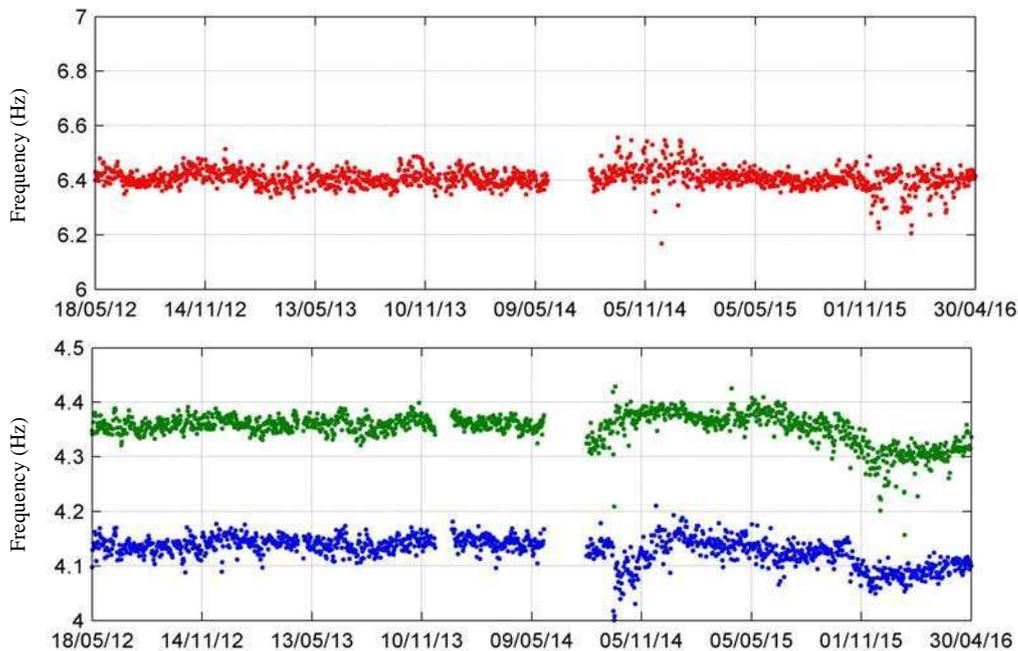
Figure 11: Time evolution of the daily average of three natural frequencies (in Hz) of the bridge from 18/05/2012 to 30/04/2016 after minimization of the temperature effect (first vertical bending mode at top and first two lateral bending modes at bottom).
