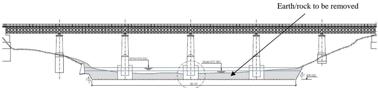
Figure 4: Retrofit of the bridge piers foundation [2].
