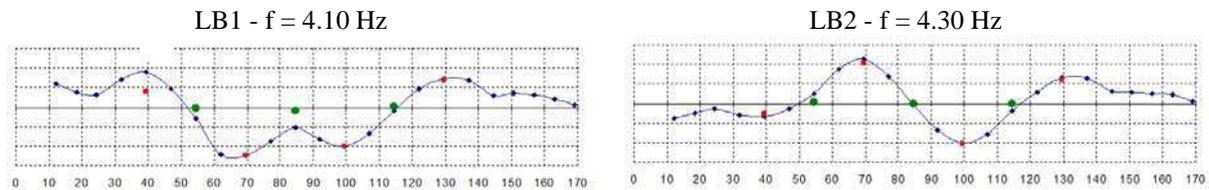
Figure 6: First two lateral bending (LB) modes
