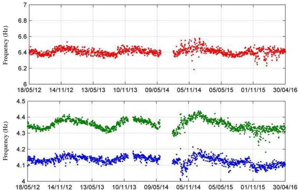
Figure 10: Time evolution of the daily average of three natural frequencies (in Hz) of the bridge from 18/05/2012 to 30/04/2016 (first vertical bending mode at top and first two lateral bending modes at bottom).
