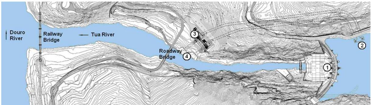
Figure 2: Location of the bridges (Roadway and Railway) and of the hydroelectric power plant components: 1-Dam; 2-Water Intake; 3-Powerhouse and Substation; 4-Outlet [1].
