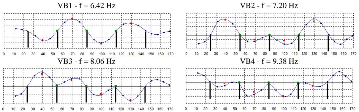
Figure 5: First four vertical bending (VB) modes
