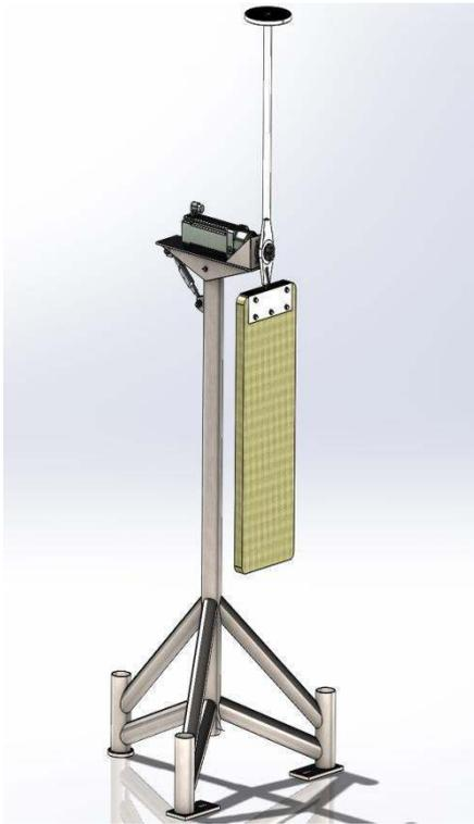
Figure 1: Laboratory rotating stage. Samples up to 70 kg can be rotated up to a frequency of 1 Hz.
