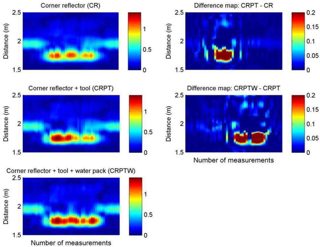
Figure 3: (left) Radargram showing different objects on the back of the GFRP-panel (corner reflector, corner reflector + tool, corner reflector + tools + water); (right) Differential analysis with adapted reference states. The respective local changes are nicely recognizable. The tool can be seen on top and the water bag at the bottom.
