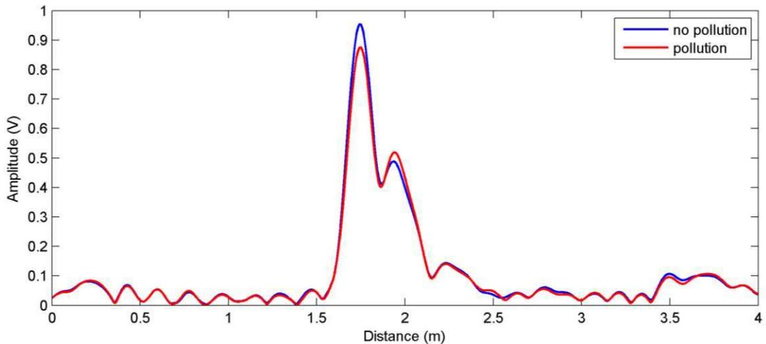
Figure 5: Comparison of a measurement with tape only and the tape with sugar. A stronger attenuation of the radar signal can be observed in the case of sugar on the rotor blade so that it seems to be possible to identify pollution on the rotor blade.
