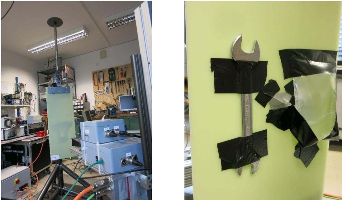
Figure 2: (left) Experimental laboratory demonstrator as a model of a wind turbine with radar module at the front; (right) different objects on the back of the 10mm thick GFR-panel (tool, corner reflector, water bag).
