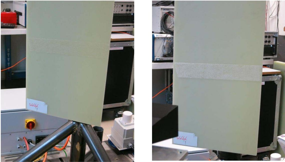
Figure 4: (left) Double-sided tape at the front side of the GFR sample; (right) Double-sided tape with sugar to simulate pollution on the rotor blades.
