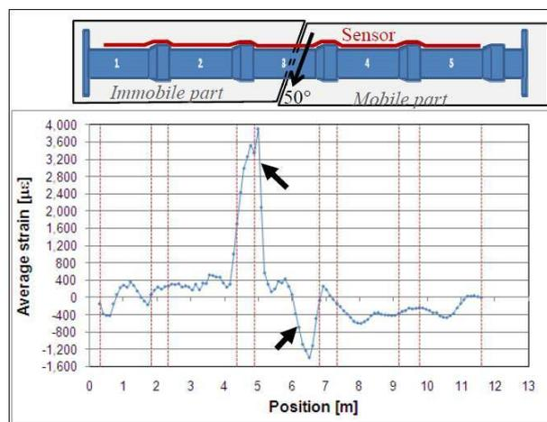
Figure 4: Sensor measurement with detected damage [25]
