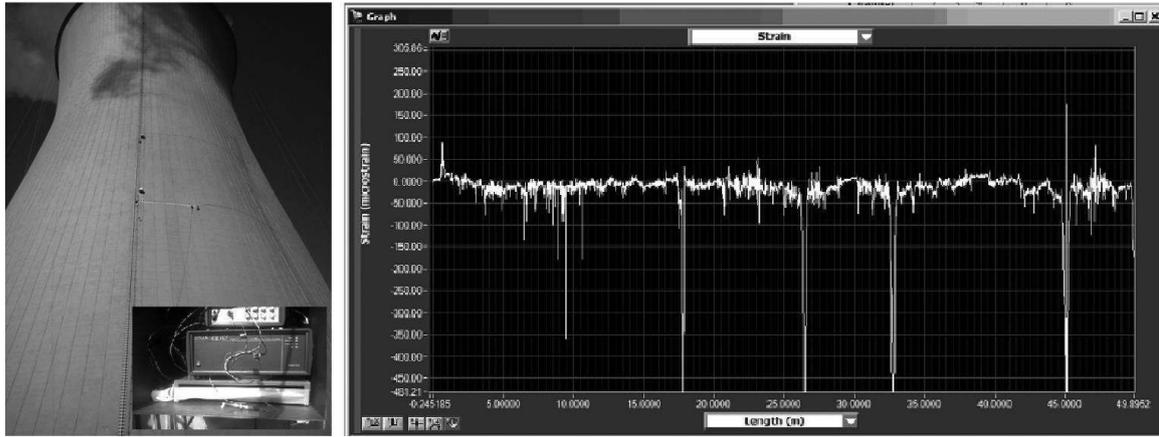
Figure 6: Instrumented concrete cooling tower (left); Strain-fiber length on the outside surface tower (right) [28]
