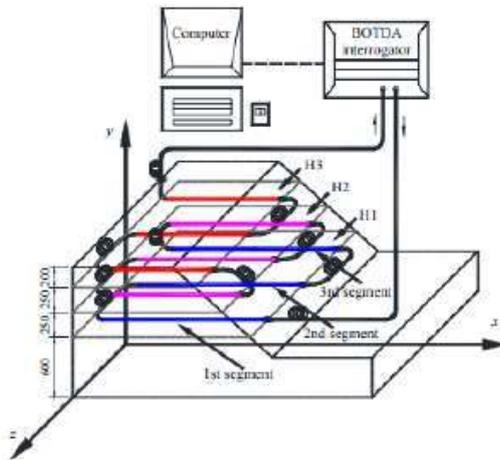
Figure 3: Layout of the BOTDA sensing fiber in the model slope (unit: mm) [23]
