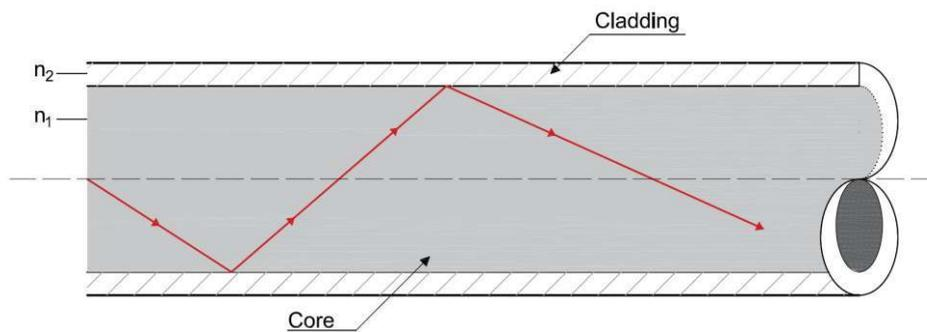
Figure 1: Light guiding and reflection in an optical fiber
