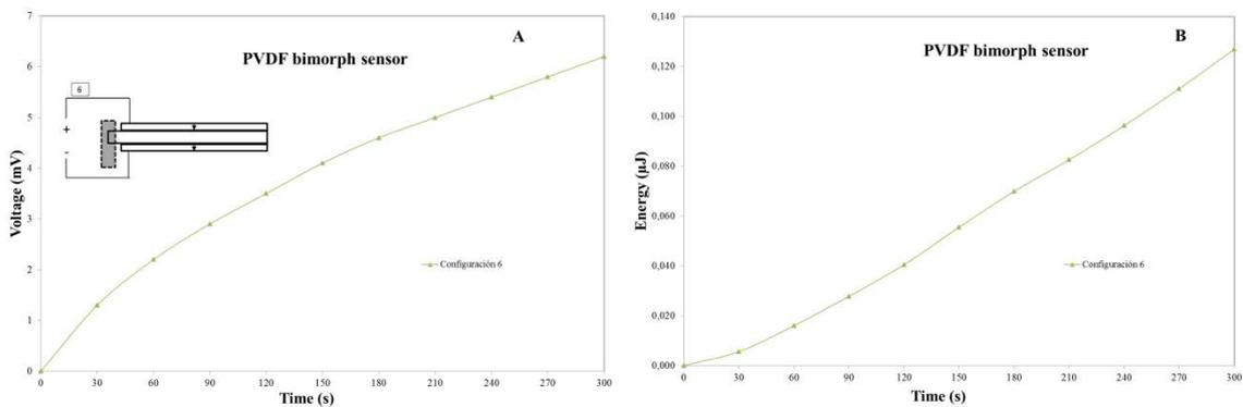
Figure 8: Voltage output (A) and Energy (B) charge history in PVDF bimorph cantilever beam sample at level 3 and 25Hz.
