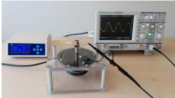
Figure 2: Shaker experimental setup.
