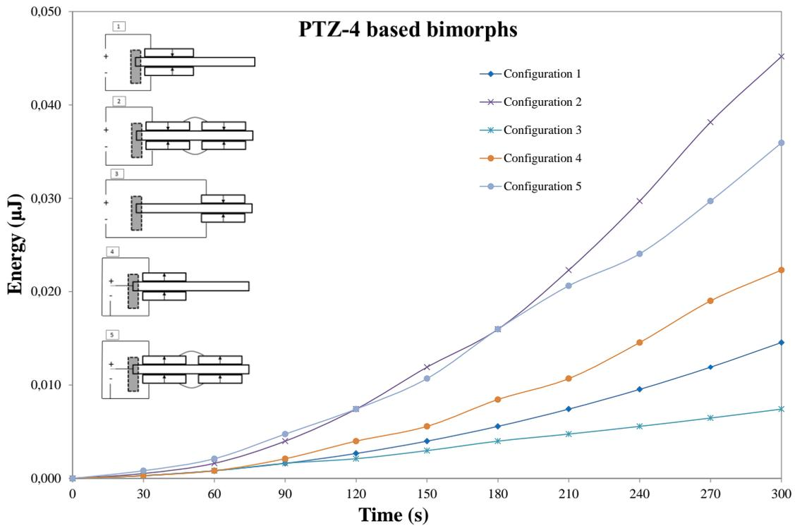
Figure 7: Energy charge history of PZT-4 bimorph samples from no.1 to 5 at level 3 and 25Hz.
