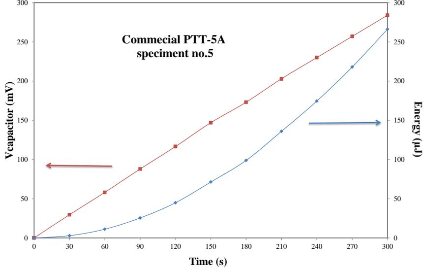
Figure 9: Voltage output (left) and Energy (right) charge history in commercial bimorph specimen.
