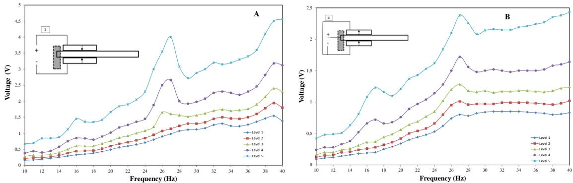
Figure 4: Open circuit voltage recorded from bimorph composed of 1 unit of PZT-4 under brass intermediate layer (A) no. 1- series connection and (B) no. 4 - parallel connection – placed near the brass tie up.
