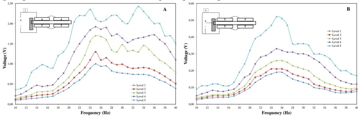
Figure 3: Open circuit voltage recorded from bimorph composed of 2 units of PZT-4 under brass intermediate layer (A) no. 2- series connection and (B) no. 5 - parallel connection.
