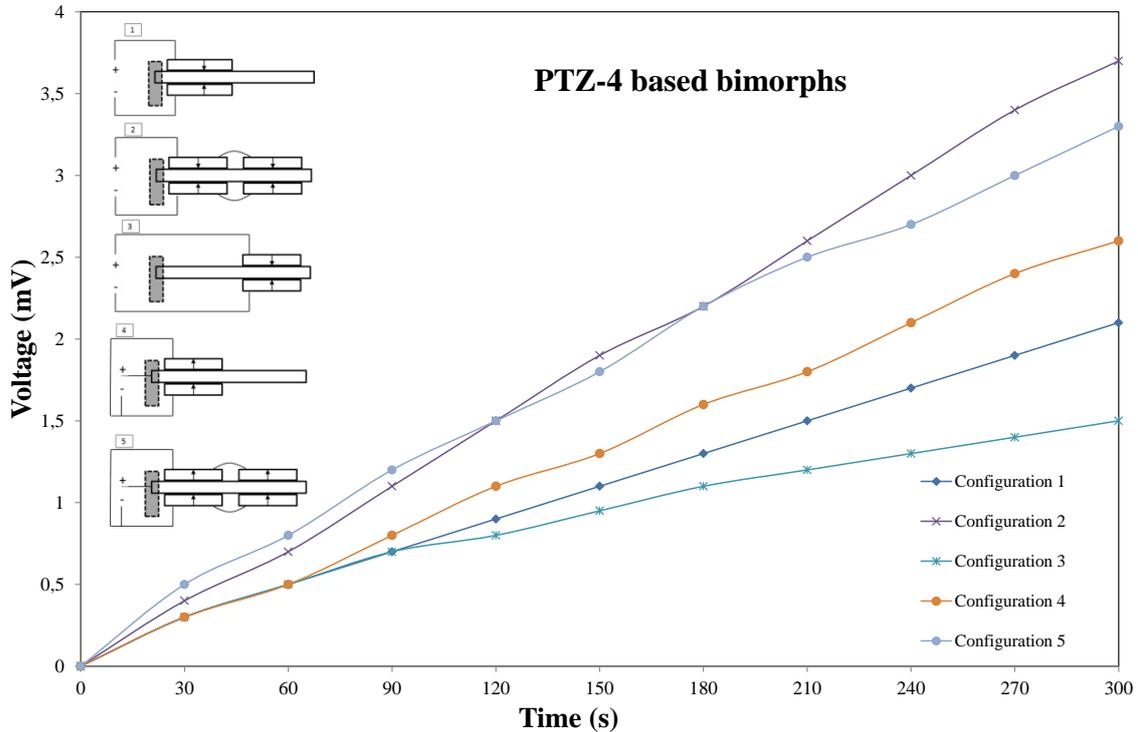
Figure 6: Voltage output charge history for samples no. 1 to 5.
