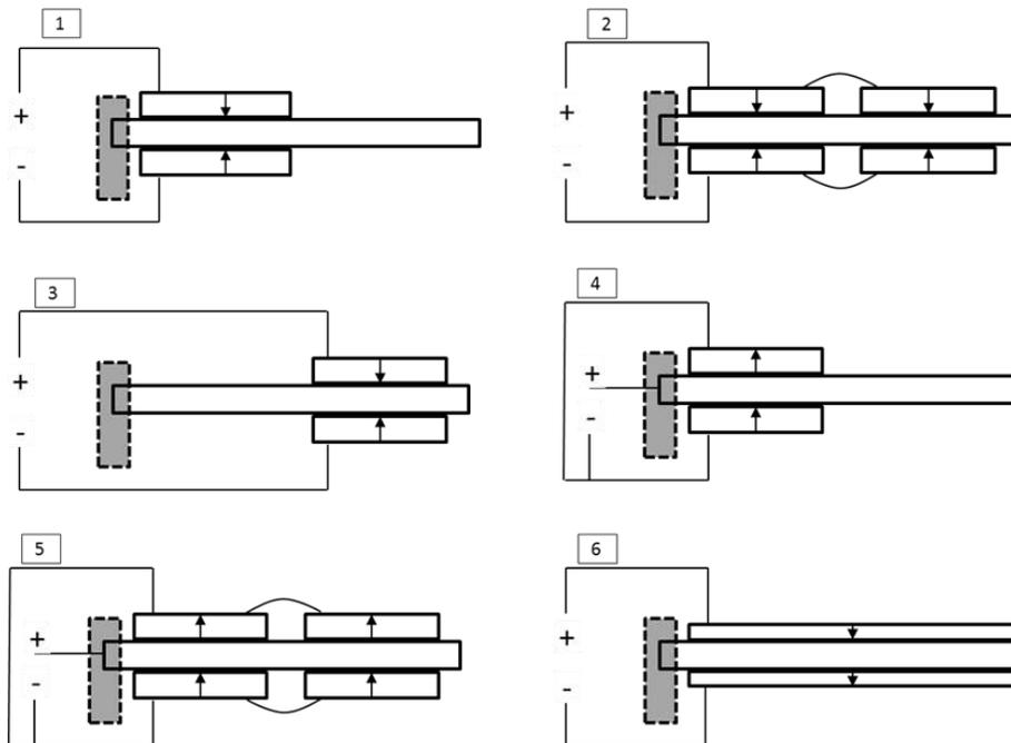
Figure 1: Bimorph schematic configurations of samples described in Table 2.
