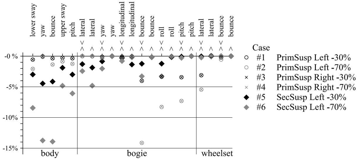
Figure 6: Changes of eigenfrequencies in different failure scenarios (>< out of phase; > in phase)
