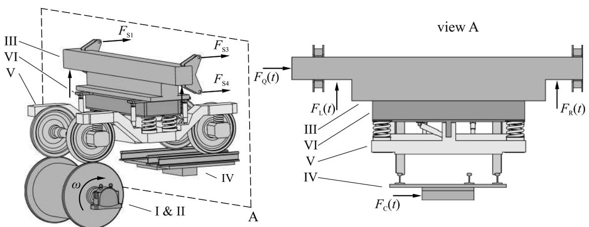
Figure 2: Concept of a 1:1 scale roller rig: drive train (I), rail roller (II), loading unit (III), curve unit (IV), test specimen (V), adapter (VI), vertical force ( $F_R$ ,  $F_L$ ), lateral force ( $F_Q$ ), curving force ( $F_C$ ), stabilizers ( $F_{S1} \dots F_{S4}$ )
