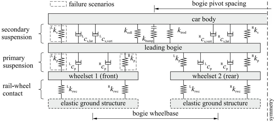
Figure 4: Topology diagram of the test train
