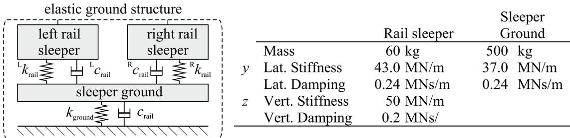
Figure 5: Topology diagram of the elastic ground
