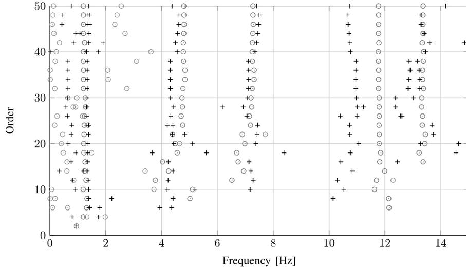
Figure 7: Results of the subspace algorithm applied to the test case (+ indicates the result for the faulty system, while o corresponds to the healthy state)
