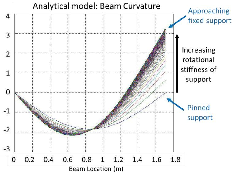
Figure 1: Analytical model for simply supported beam with increasing rotational stiffness of right beam support.
