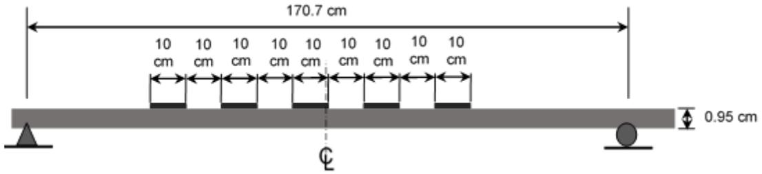
Figure 3. Simply supported aluminum beam dimensioning and FBG sensor positions [8].
