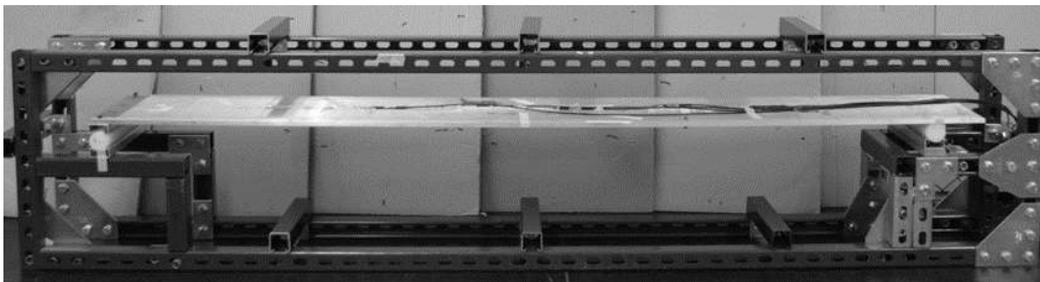
Figure 2. Simply supported aluminum beam used in experimental testing [8].
