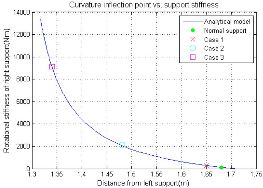
Figure 5: Experimental inflection points corresponding rotational stiffness of support based on analytical model.
