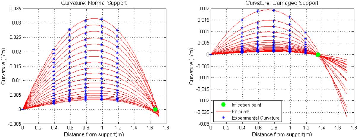
Figure 4: Curvature mode fitting for undamaged and damage laboratory tests.
