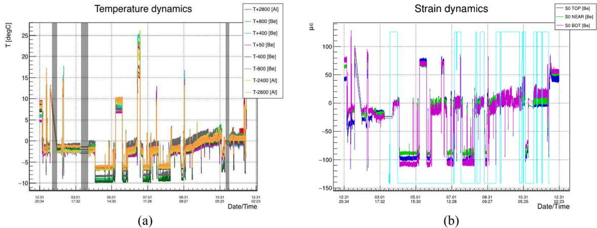
Figure 5: Temperature profile of the beam pipe (a) and behaviour of the strain acting on the beam pipe during different phases of switching on and off of the magnetic field recorded during different magnet test periods (b), during the CMS operation throughout 2015. The cyan line represents the B-field variation from 0 to 3.8 Tesla.
