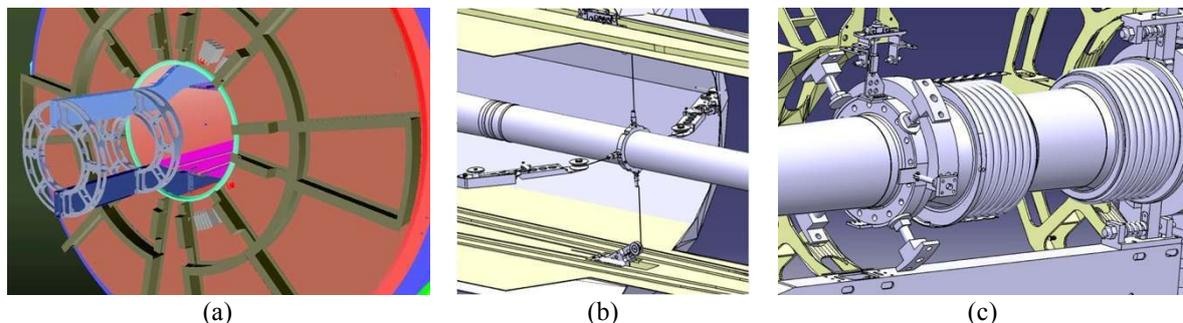
Figure 4: Technical drawing of: the permanent supports for the central beam pipe and bellows attached to the tracker bulkhead, (a); the x-y support for the central pipe for tensioning and regulation, (b); the bellows between the central and the endcap beam pipe sectors, (c).
