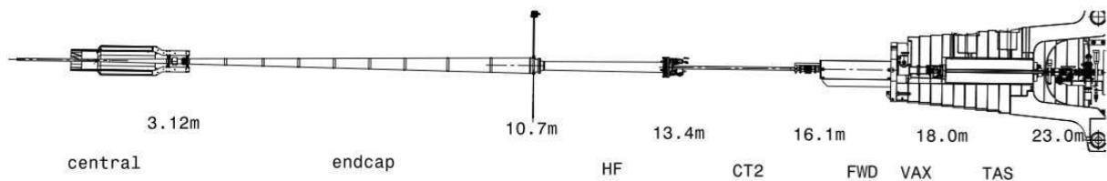
Figure 3: Drawing of one side, with respect to the impact point, of CMS beam pipe. Different sectors are shown.
