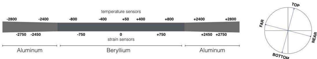
Figure 2: Layout of the fiber optic monitoring system installed on the CMS central beam pipe. 4 FBGs array are installed and on each array there are 16 FBGs: 7 configured as strain and 9 as temperature sensors.
