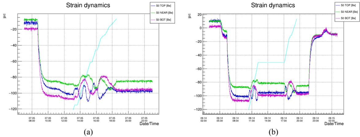
Figure 6: Strain behaviour on the central part of the pipe during the B-field rump performed on July, 7<sup>th</sup> 2015 (a) and on September, 14<sup>th</sup> 2015 (b). The cyan line represents the B-field variation from 0 to 3.8 Tesla.
