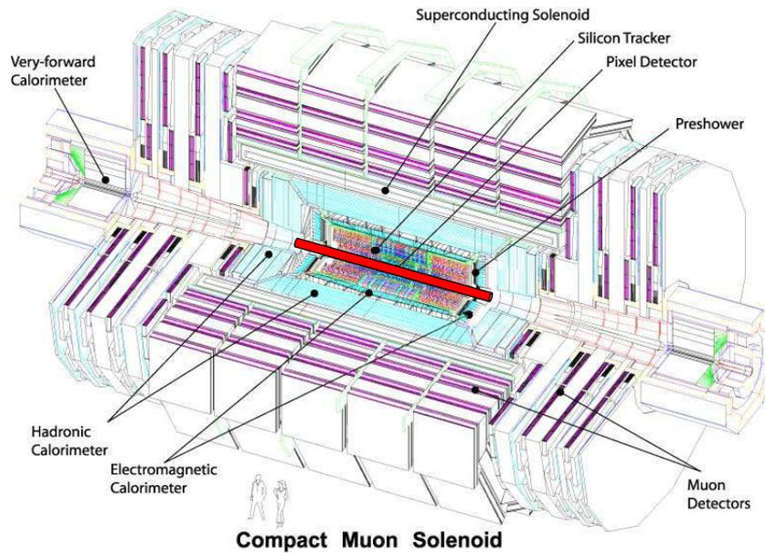
Figure 1: CMS detector technical view. All the subdetector are labelled: pixel, silicon tracker, ECAL, HCAL, superconducting solenoid, iron return yoke with muon chambers. The monitored Pipe is the LHC section located into CMS, here colored in red.
