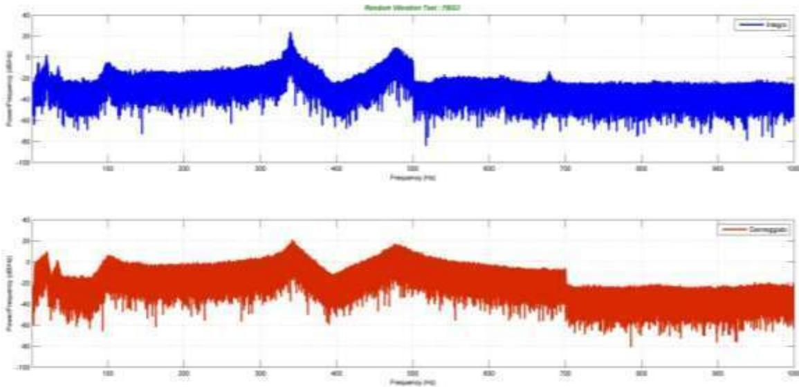
Figure 7 – Random vibration spectra for pristine and impacted component recorded on FBG4 sensor
