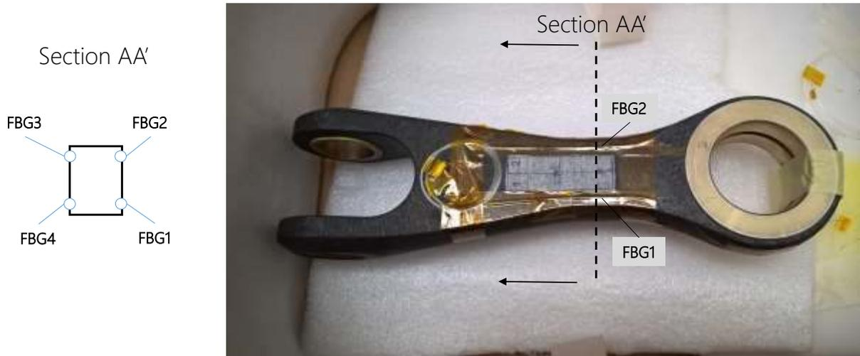
Figure 2 – FBG installation on composite drag link
