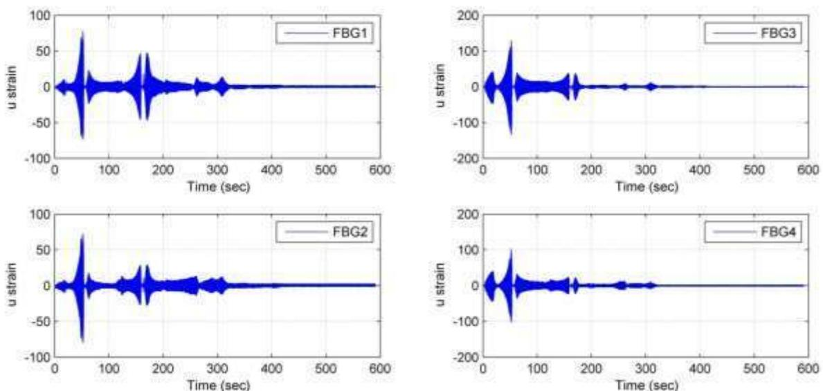
Figure 4 – Strain history during sine sweep test
