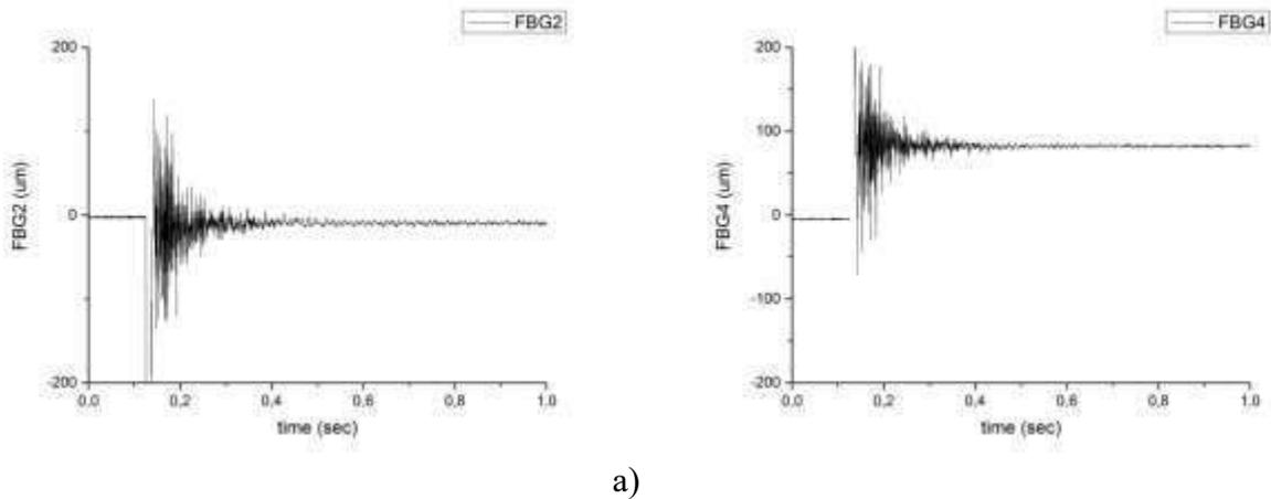
Figure 5 – Deformation recorded during the impact test. a) sensor on the impacted side, b) sensor on the opposite wedge
