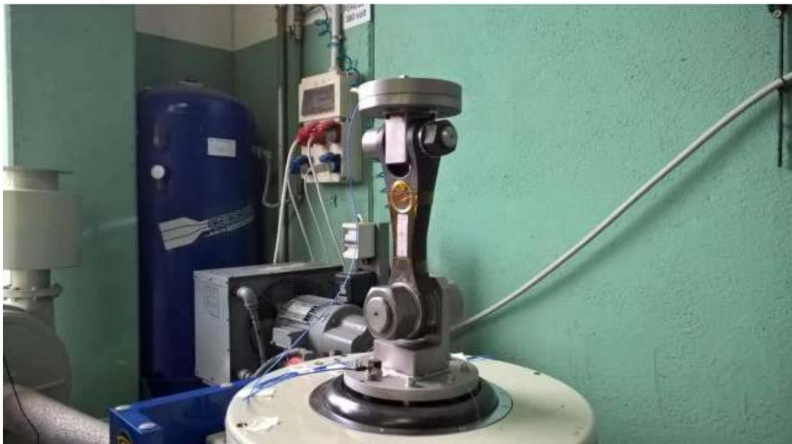
Figure 1 – Experimental test set-up
