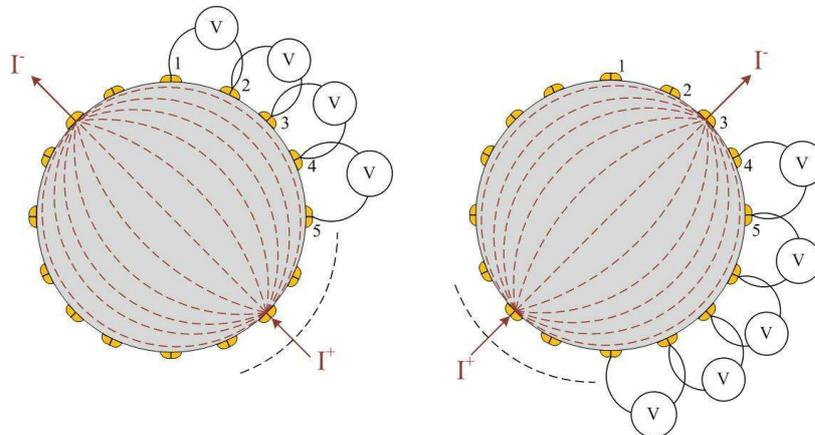
Figure 1: Schematic illustration of EIT measurements corresponding to two current injections.
