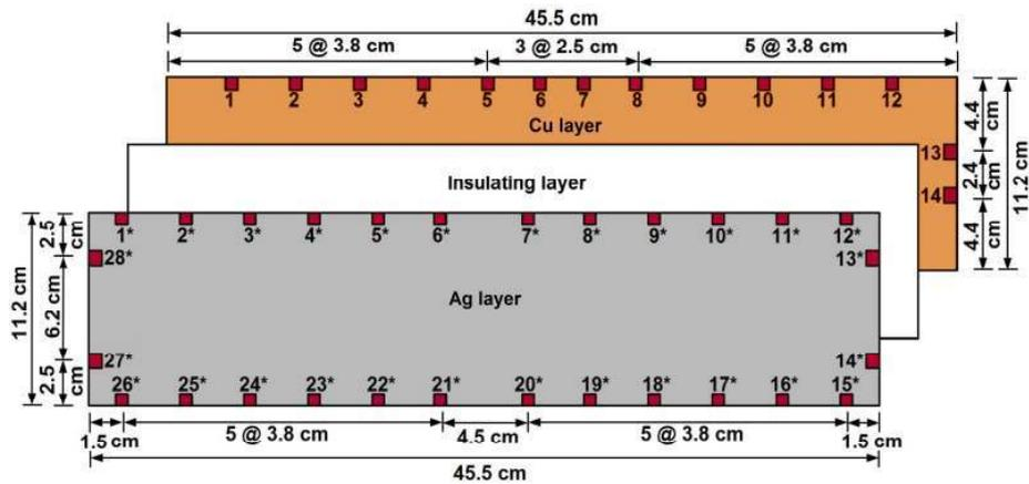
Figure 5: Schematic illustration of the multi-layer sensing skin applied on the surface of a concrete beam.
