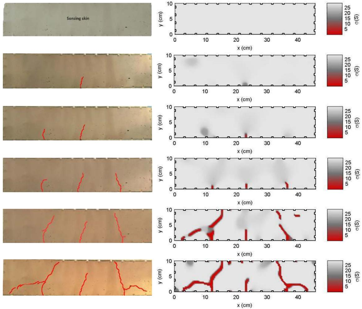
Figure 4: Single layer sensing skin applied on a concrete beam surface; photographs of the sensing skin (left column) and EIT reconstructions of the sensing skin (right column).
