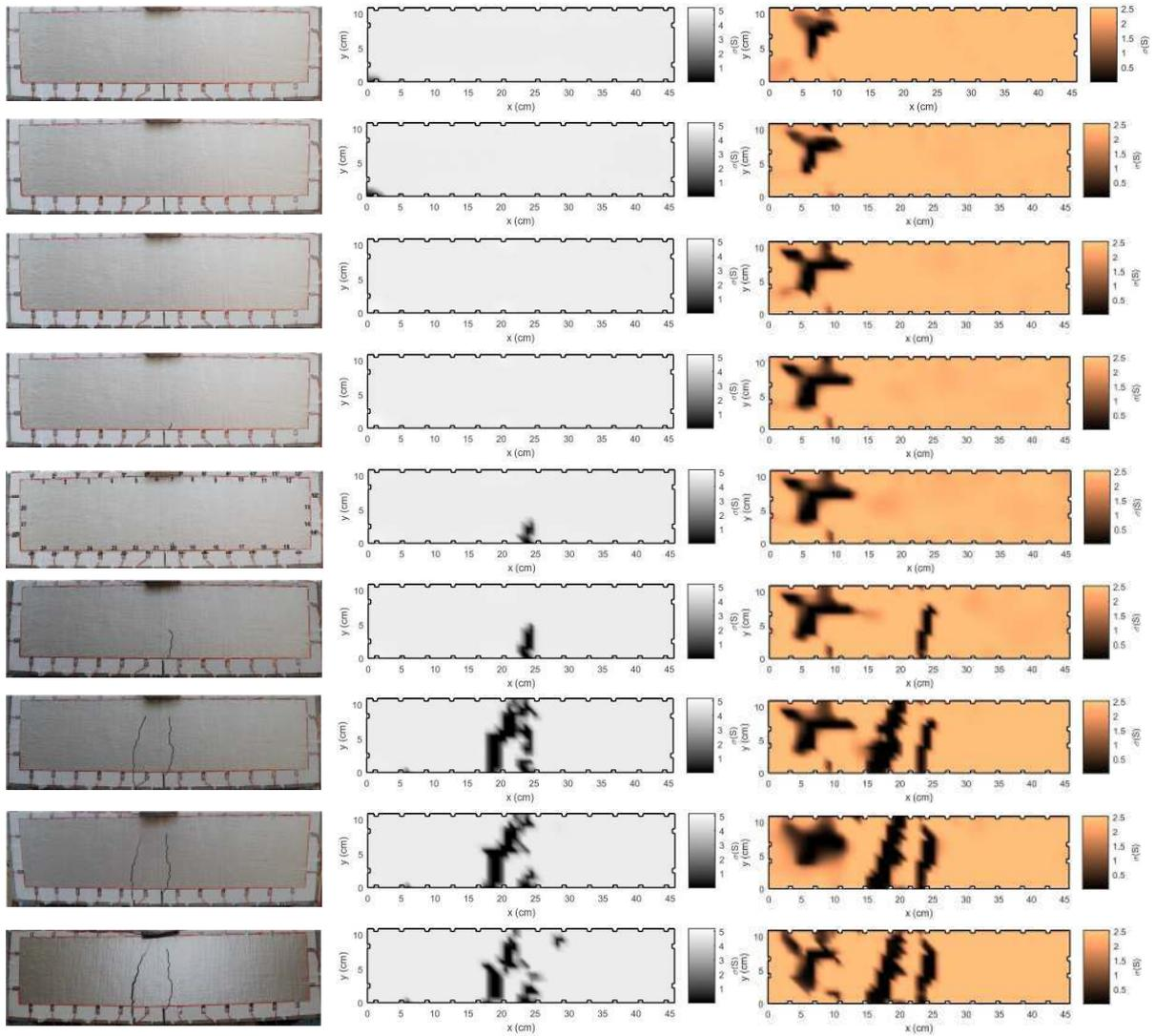
Figure 6: Photographs of the sensing skin at times of EIT measurements (left column), and the corresponding EIT reconstructions of the Ag [crack detection] layer (middle column) and the Cu [chloride and crack detection] layer (right column). The first four lines correspond to times 12, 24, 96 and 144 hours of chloride solutions ingress, and the last five lines correspond to three-point bending at load levels 11.6, 16.9, 27.6, 23.1 and 21.8 kN.
