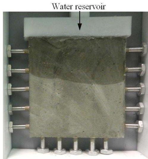
Figure 2: Imaging of moisture flow with EIT. Photograph of the specimen 60 minutes after adding water.
