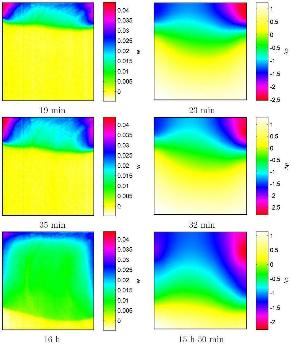
Figure 3: Imaging of moisture flow; neutron radiography images (left column) and EIT reconstructions (right column). The times of the neutron exposures/ERT measurements are shown under the images.
