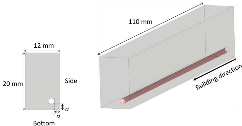
Figure 1: Cross-section of the capillary ( $a = 1.8$  mm) positioned at distance  $a$  from the specimen's surface.
