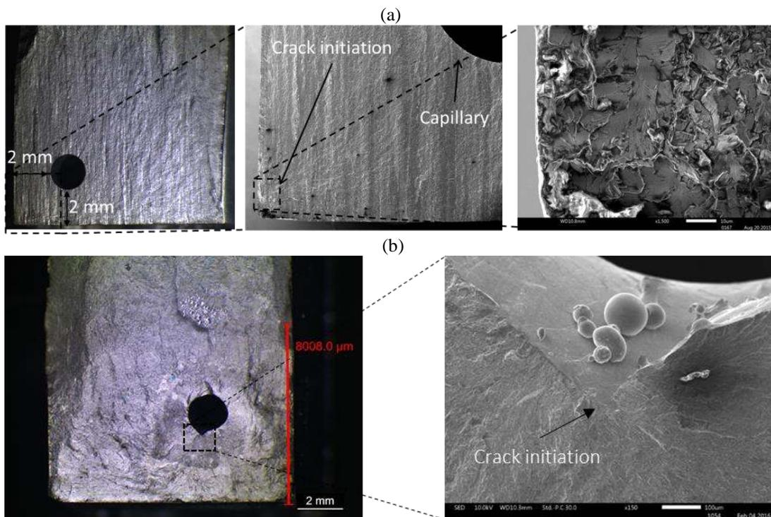
Figure 5: Scanning electron microscopy images of the cross-sections of the fracture surface of (a) a conventional Ti6Al4V specimen where the crack nucleated from the edge of the specimen and (b) an LMD autofrettaged sample with 3 mm capillary location with crack nucleation location at the capillary region.
