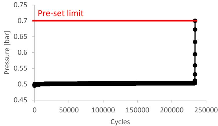
Figure 4: Pressure vs. total cycles during the fatigue life of an annealed LMD specimen.
