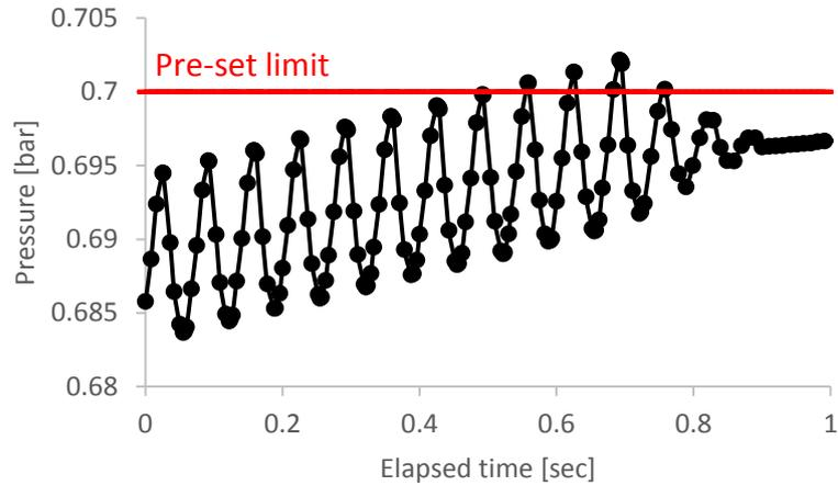
Figure 3: Pressure vs. elapsed time for an annealed LMD specimen during the last second of the fatigue test.
