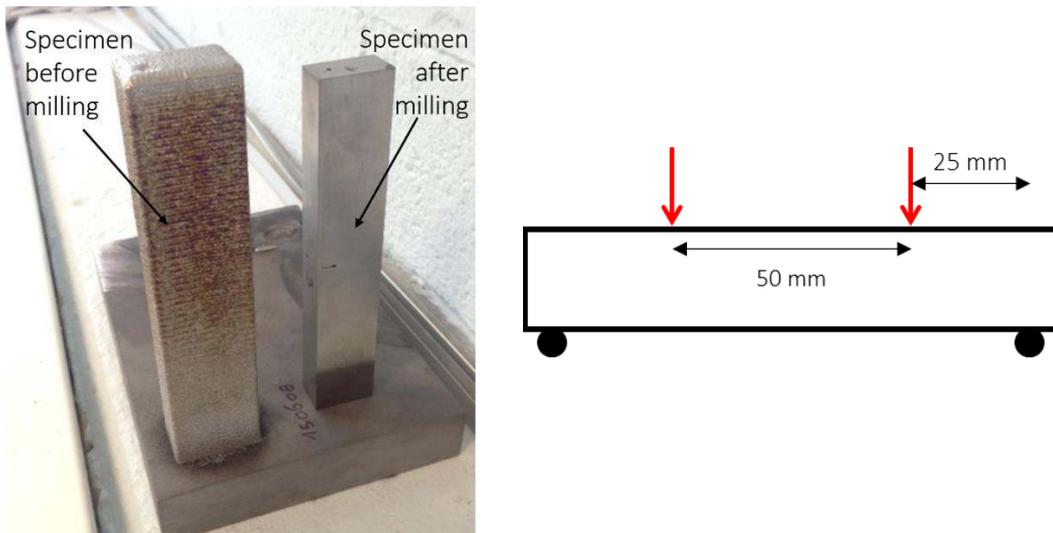
Figure 2: (a) Specimen after the LMD production and final specimen after machining. (b) Schematic representation of four-point bending setup.
