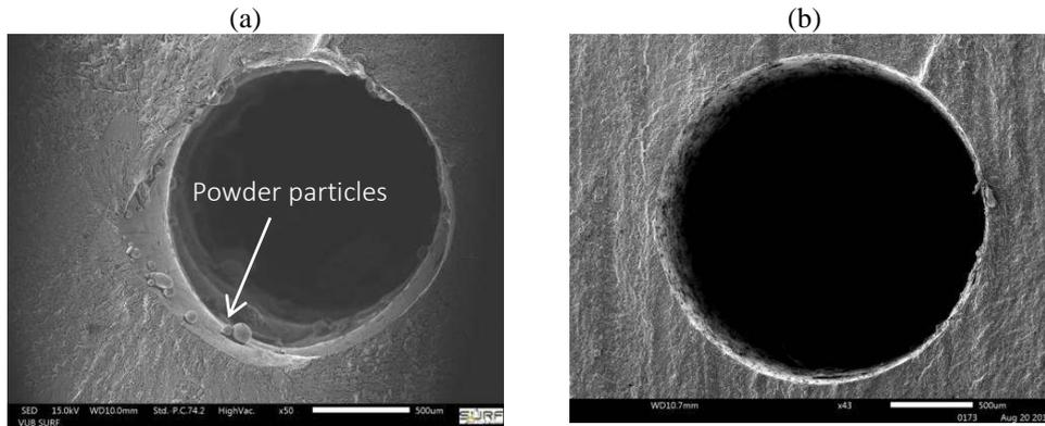
Figure 6: Capillary region of Ti6Al4V (a) produced by laser metal deposition with high roughness and (b) capillary produced by gun drilling on the conventional specimen with a fine surface finishing.
