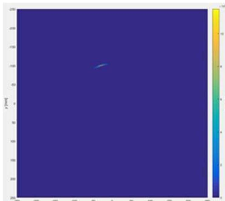
Figure 11: Experimentally obtained B-Mode image for a CFRP plate with a hole
