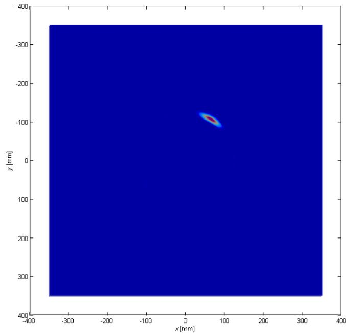
Figure 7. B-Mode image maximizing the A0 mode (50 kHz)
