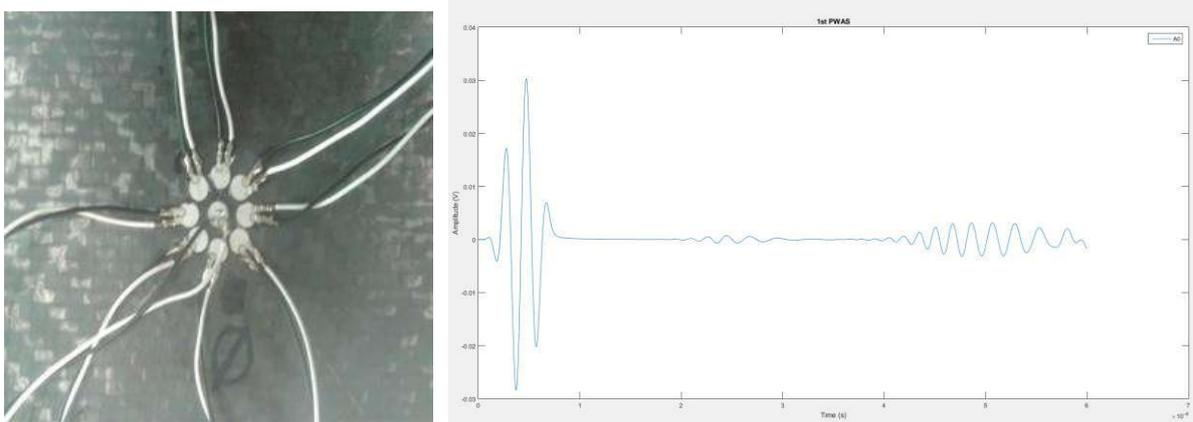
Figure 10. PWAS STMR ring topology (left) and signal measured by a receiver PWAS (right)
