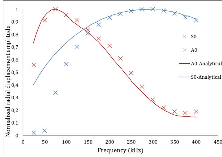
Figure 4: Normalized radial displacement amplitudes of the piezo-plate response.
