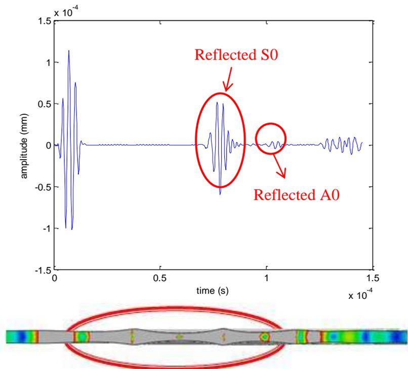
Figure 8. Reflection bursts for a 375 KHz excitation that maximizes the S0 mode (above) and plate section showing the generated symmetric S0 mode (below)
