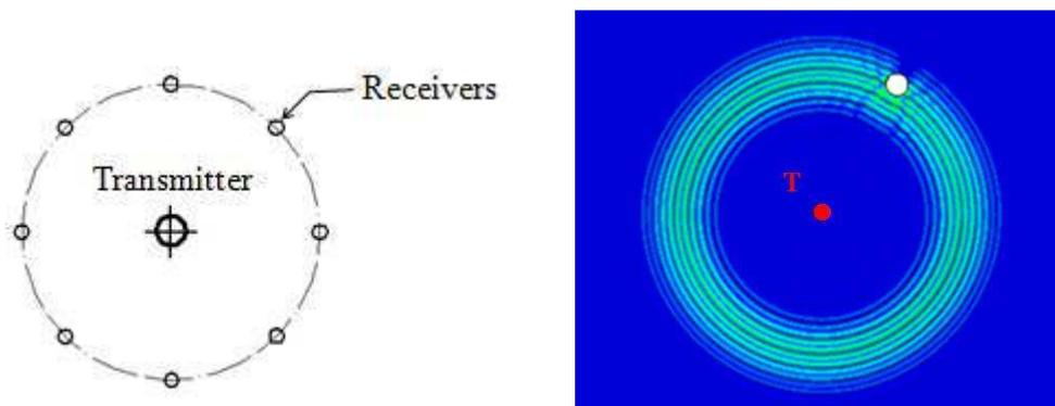
Figure 1: STMR ring topology (left) and wave front radiated by the transmitter PWAS (right)
