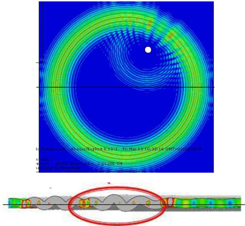
Figure 5: Wave front for a 50 kHz excitation (above) and plate section showing the generated antisymmetric A0 mode (below)
