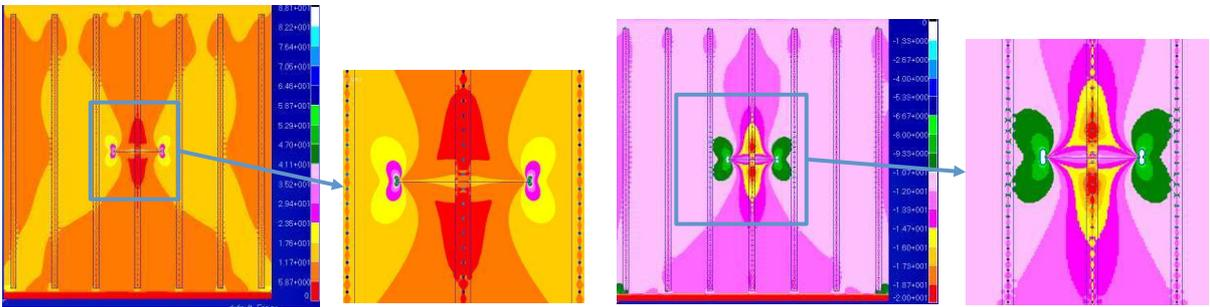
Figure 3: Simulation of a stiffened panel with a crack in terms of stress distribution (left) and probability of damage (right)
