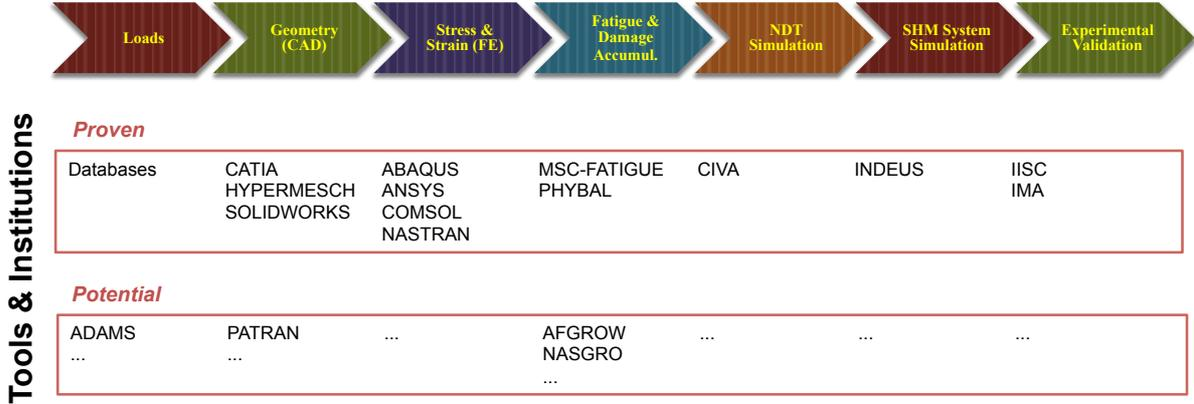
Figure 1: SHM validation and verification process chain
