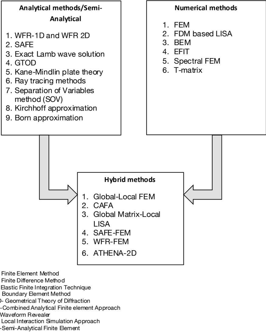
Figure 5: Hybrid methods for guided wave SHM modeling
