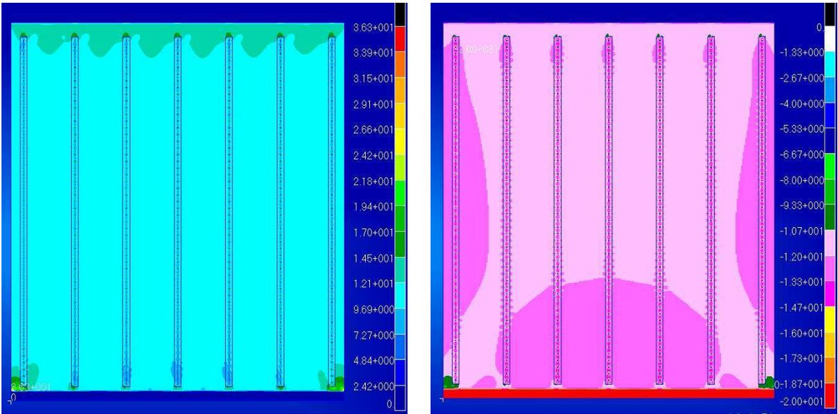
Figure 2: Simulation of a stiffened panel in terms of stress distribution (left) and probability of damage (right)
