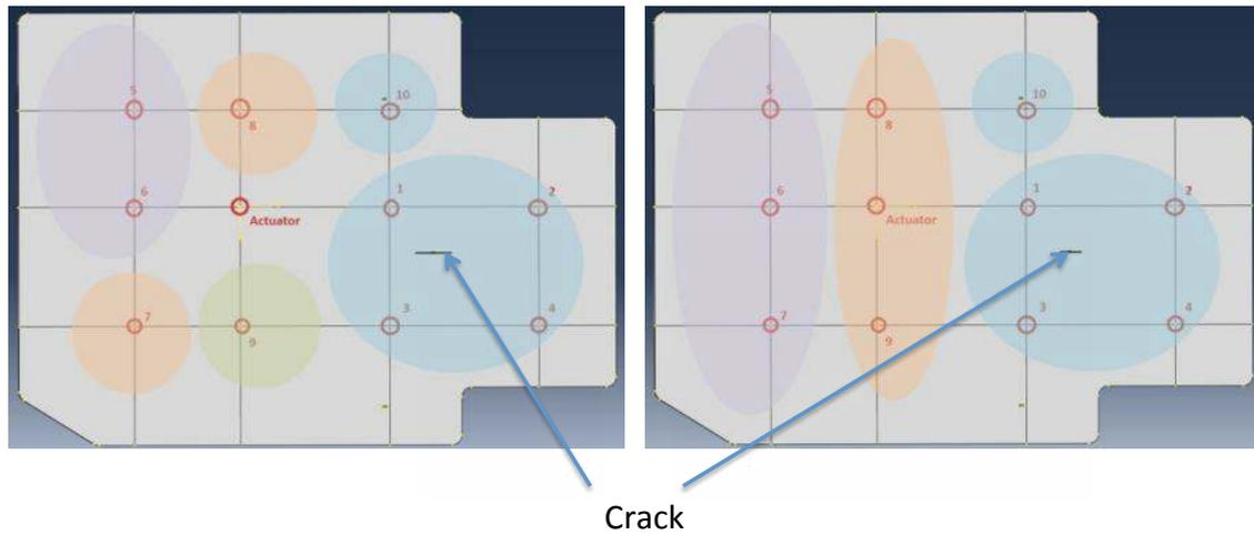
Figure 7: Detectability map of cracked panel: 20 mm long crack (left) and 12 mm long crack (right)
