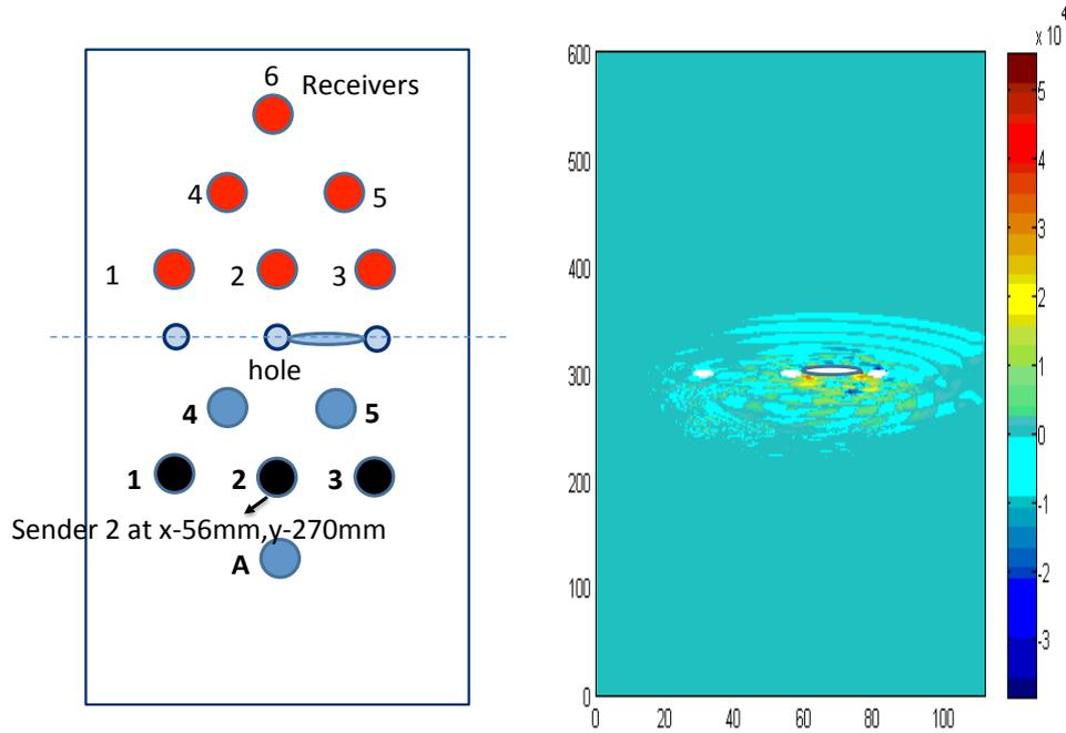
Figure 6: Three hole aluminium plate with crack: transducer configuration with three actuators used shown in black (left) and resulting guided wave differential plot (right)
