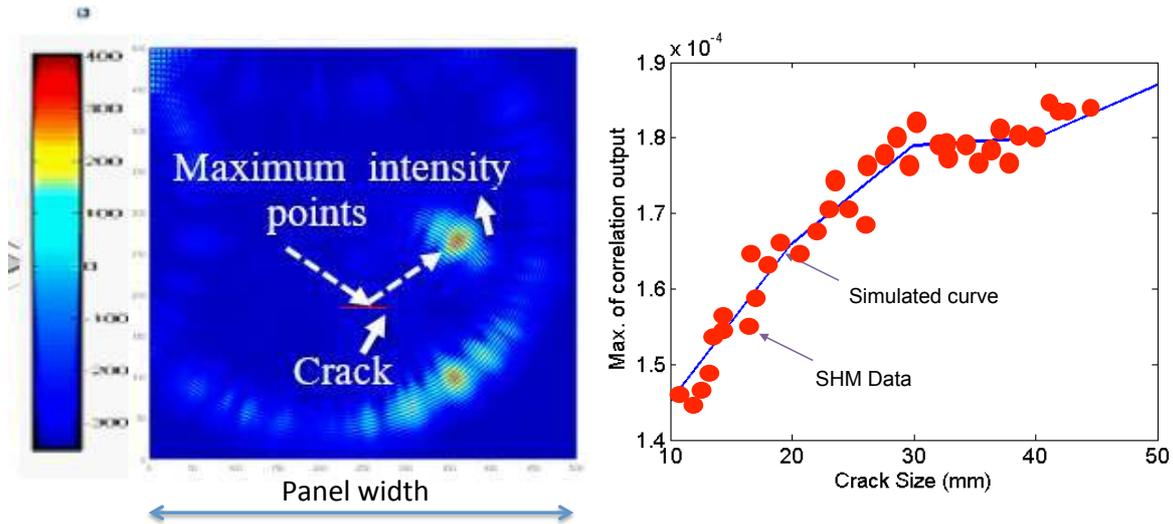
Figure 8: Simulation results for stiffened aluminium panel: Differential plot for transducer location placement (left) and online experimental verification of simulated crack propagation curve (right)
