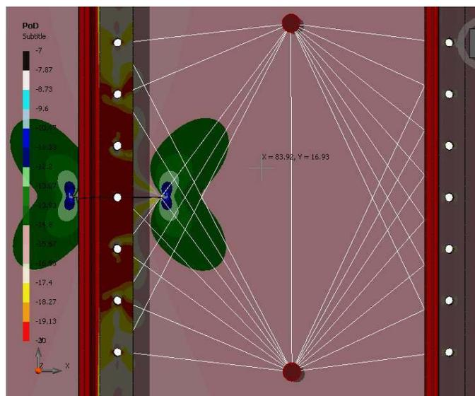
Figure 4: Guided wave transmitter and receiver placement analysis based on ray tracing
