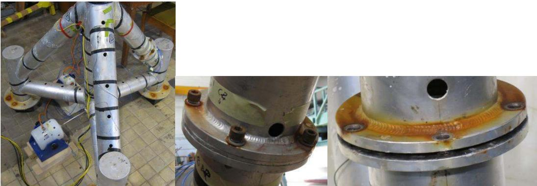
Figure 1 Instrumented tripod structure for the acceleration and strain measurements (left), with model of the circumferential crack in partial open (center) and total failure (right) configurations of screwed flanges.
