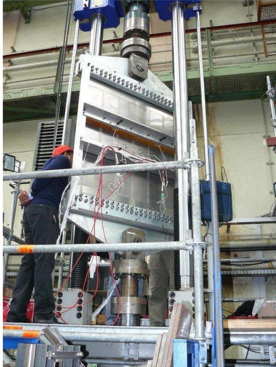
Fig 6. Test set-up at IMA Dresden. Instrumented stiffened panel under fatigue loading is shown
