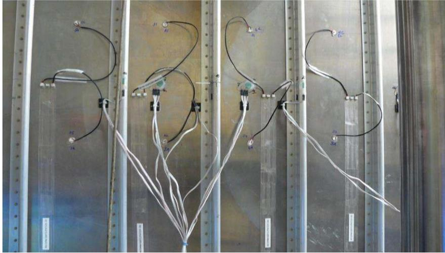
Fig 8. Piezo-electric sensors and strain gauges mounted on test panel
