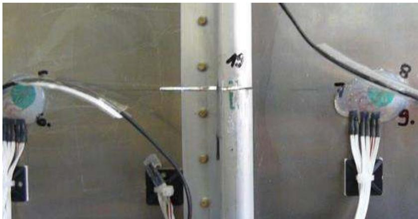
Fig 7. Introduction of initial crack of 50mm length
