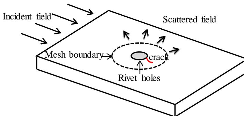
**Fig.2 Finite element mesh on the rivet holes**
