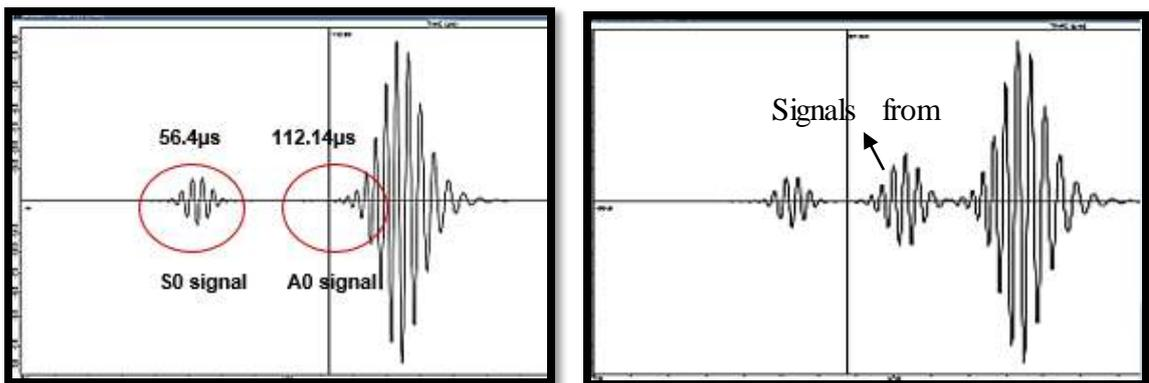
Fig. 14 Results of guided wave using CIVA-GWT module
