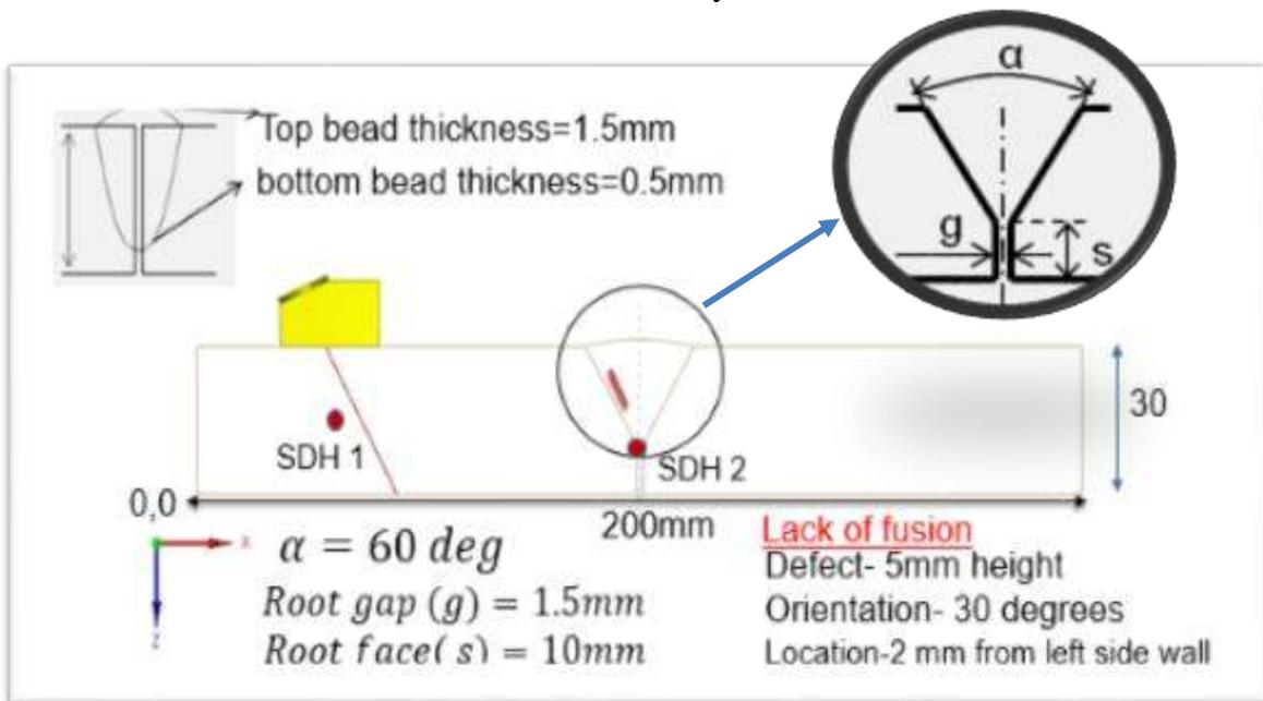
Fig.6 Weld geometry model for bulk wave validation .
