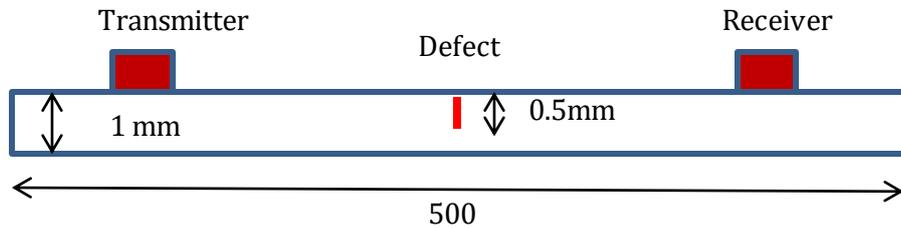
Fig. 13 Guided wave validation model of a rectangular plate
