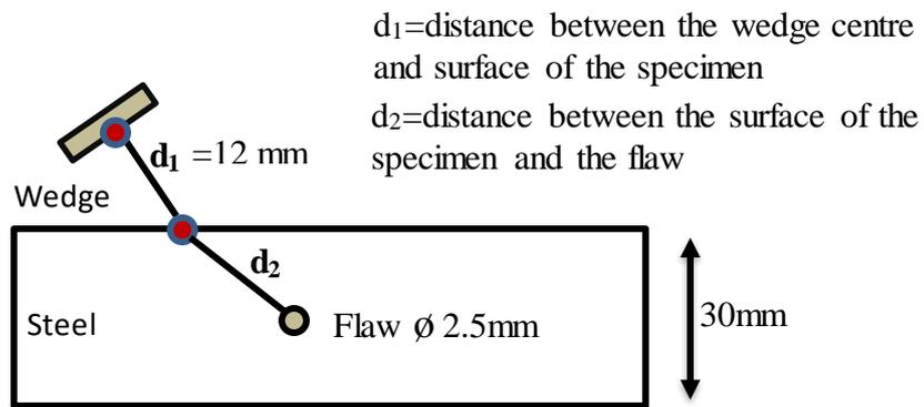
Fig 8. Travel time computation for angle beam inspection of 45°
