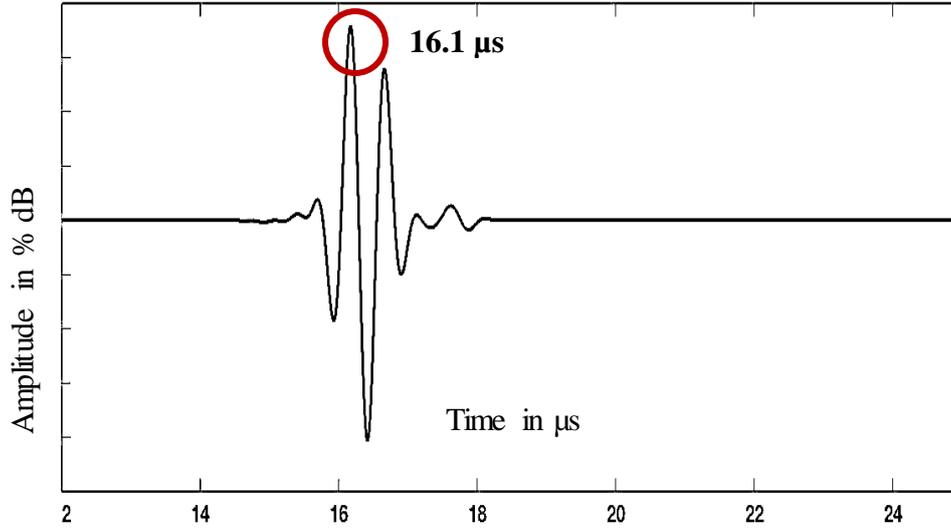
Fig 9. A scan at the target of angle beam inspection of 45°
