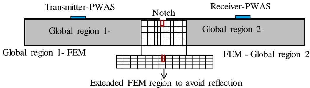
**Fig. 4 Global-local FEM approach using PWAS patches**
