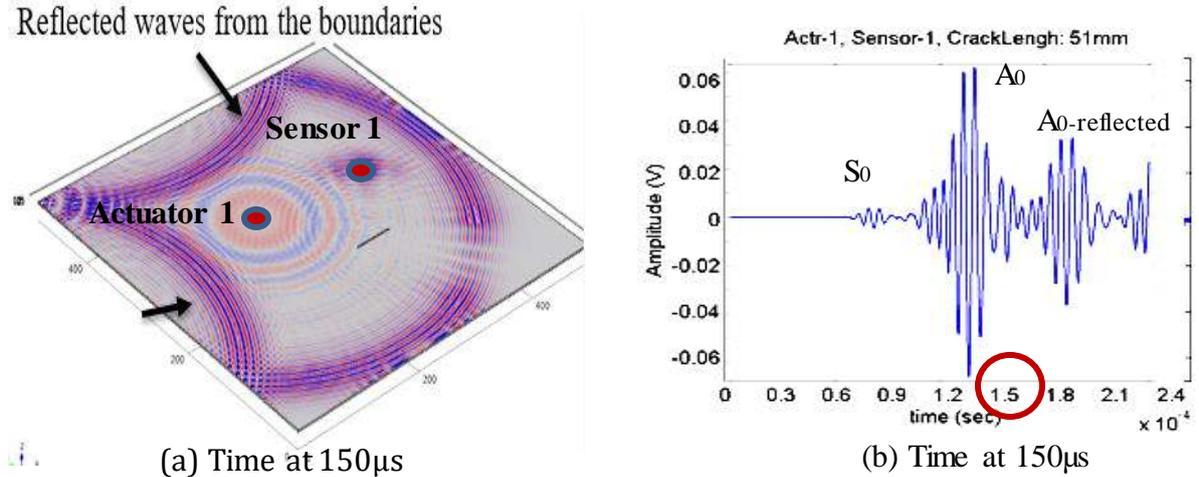
Fig.12 Guided waves results from COMSOL simulation and raytracing module from IN-DEUS
