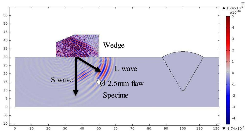
Fig 10. Bulk wave propagation using COMSOL-Multiphysics
