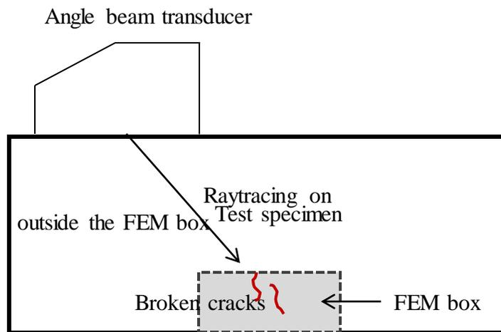
**Fig.2 ATHENA 2D combines Raytracing outside and FEM inside the box.**
