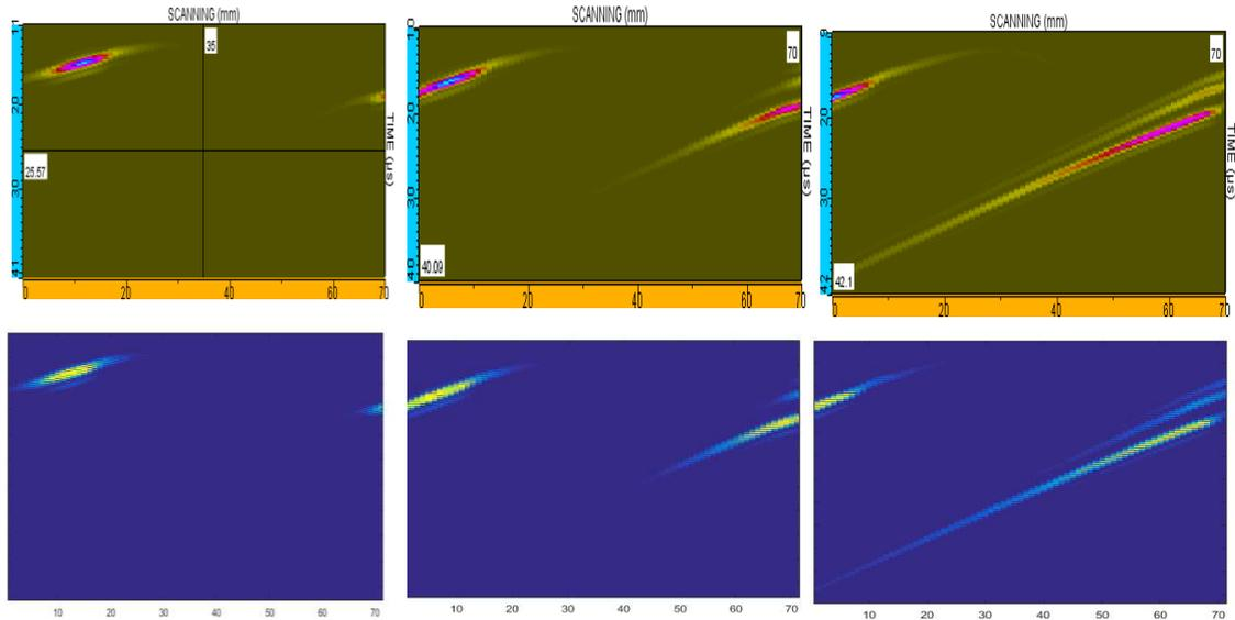
Fig 7. B-scan results for 30°, 45° and 60° angle of inspections using CIVA and raytracing tool
