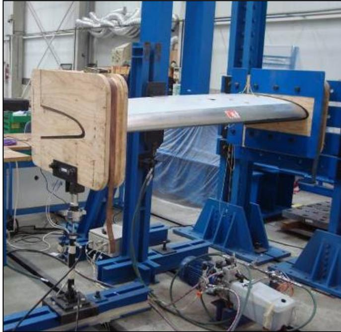
Figure 2: Demonstrator developed in AIRHEM-08. Leading edge of a wing instrumented with SHM.
