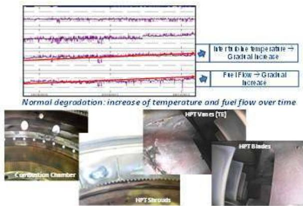
Figure 11: performance evolution and component status under normal operation
