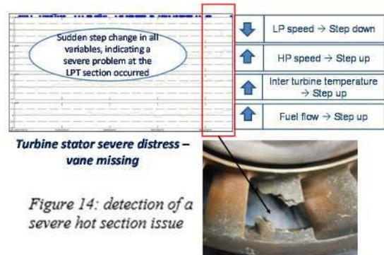
Figure 14: detection of a severe hot section issue
