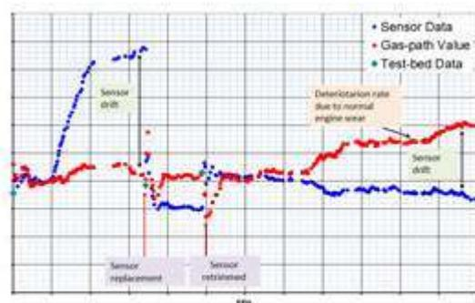
Figure 13: sensor temperature and gas path derived Temperature evolution with EFH
