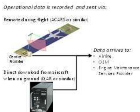
*Fig. 9: operational data recording and transmission*
