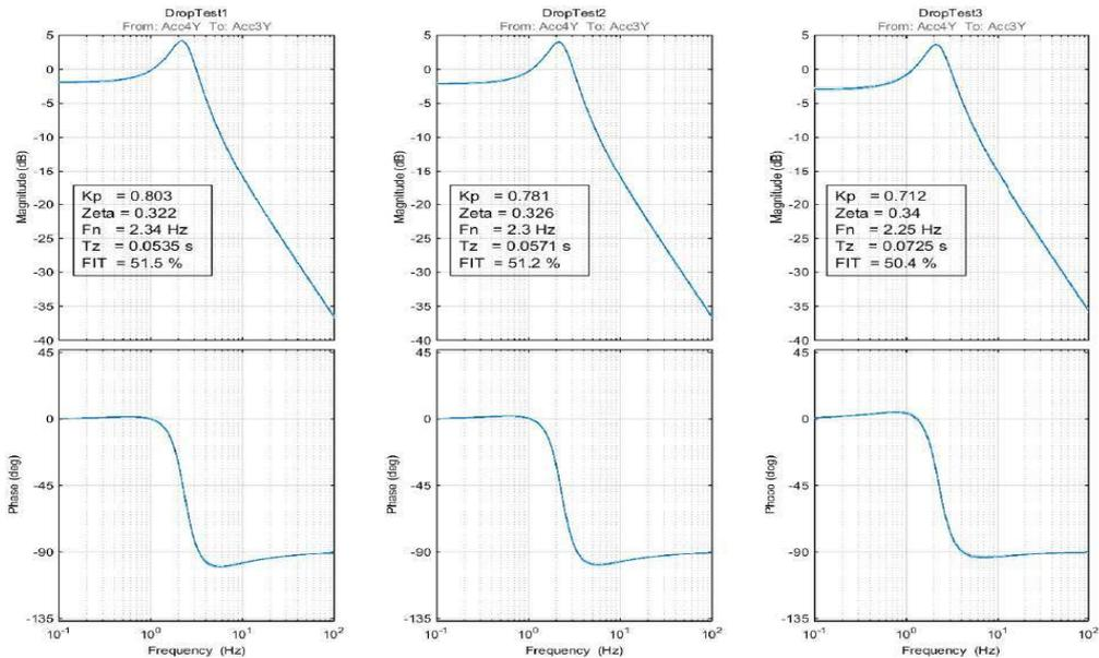
Figure 5: Bode diagrams of different drop tests.
