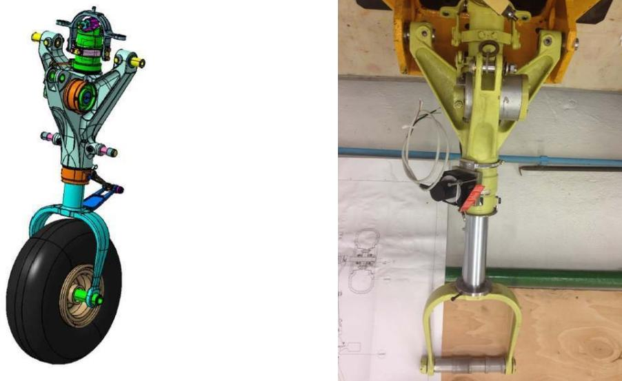
Figure 2: Landing gear test article.
