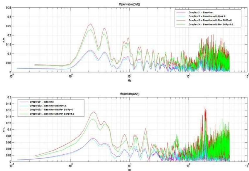
Figure 6: DFT diagrams of time domain derived data from the two sensors (up: on the tire support and down: on the airplane-landing gear support connection) with modified pressure in the landing gear shock absorber and tire.
