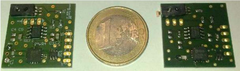
Figure 1. RFID sensor system (UHF left, HF right)
