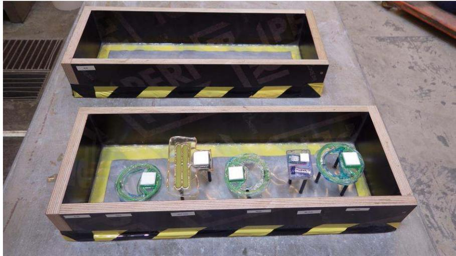
Figure 3. Test specimen with RFID systems before filling with concrete.
