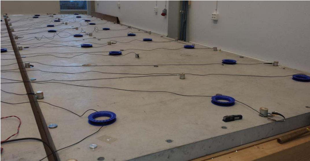
Figure 1: Photograph of the monitored concrete floor slab and the piezoelectric transducers used for measurements.
