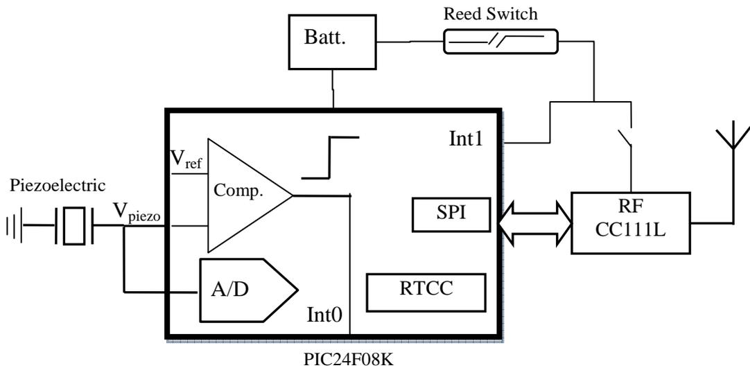
Figure 1. Impact detection, sensor subsystem block diagram.
