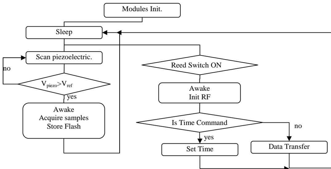
Figure 2 Operations sequence flow diagram. Sensor subsystem.
