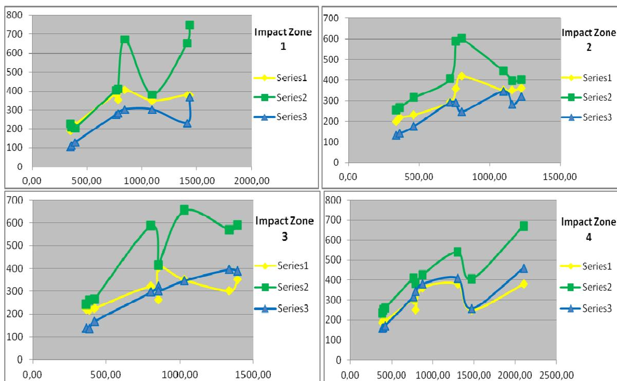
Figure 7. Peak voltage amplitudes vs impact forces for the three sensors for the four different zones of impact made on composite material. Horizontal axe: force of the impact in Newtons. Vertical axe: peak voltage of the signal in millivolts.
