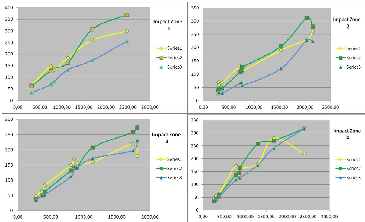
Figure 6. Peak voltage amplitudes vs impact forces for the three sensors for the four different zones of impacts made on aluminum plate material. Horizontal axe: force of the impact in Newtons. Vertical axe: peak voltage of the signal in millivolts.
