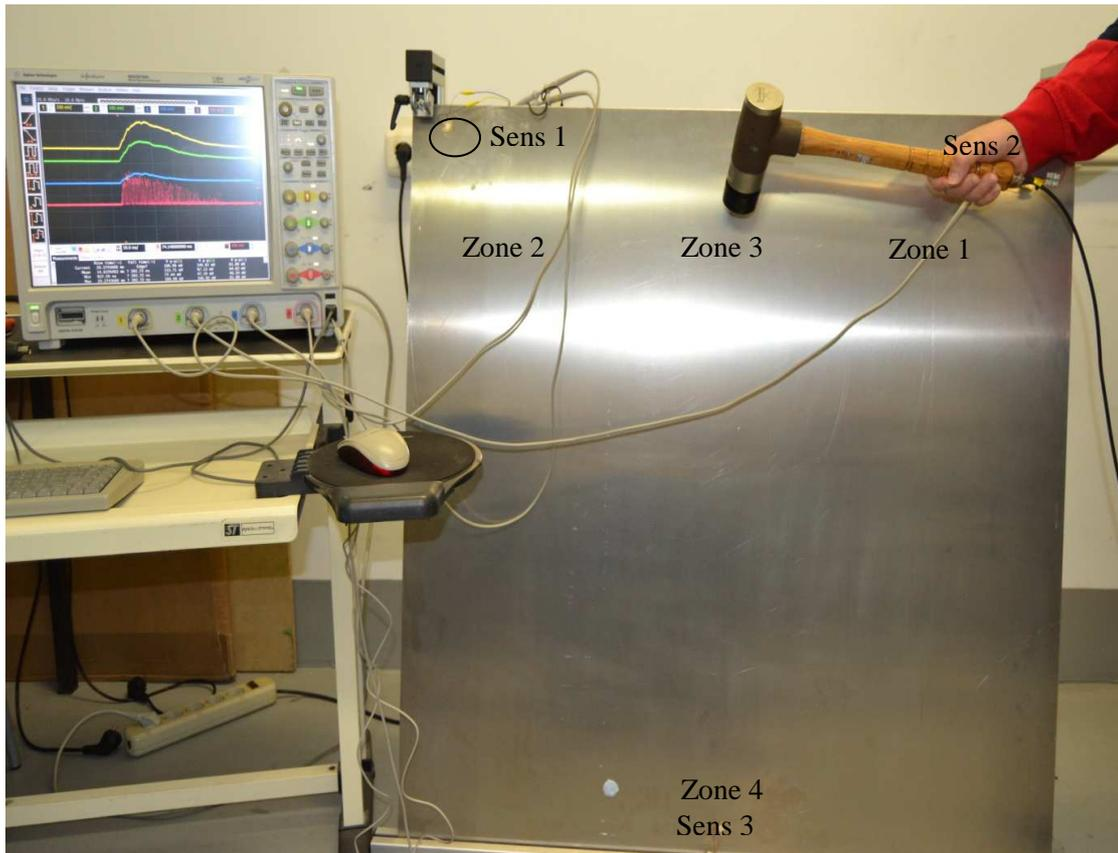
Figure 4. Picture of the experimental setup.
