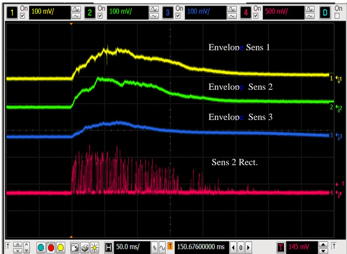
Figure 5. Oscilloscope signals showing voltages of envelope and rectified signals from the three transducers.
