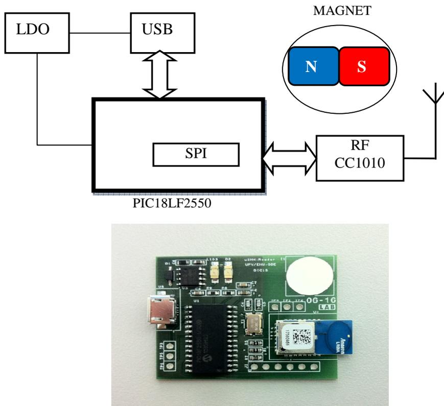
Figure 3. Top: Impact detection, reader subsystem block diagram. Bottom: reader electronic card.
