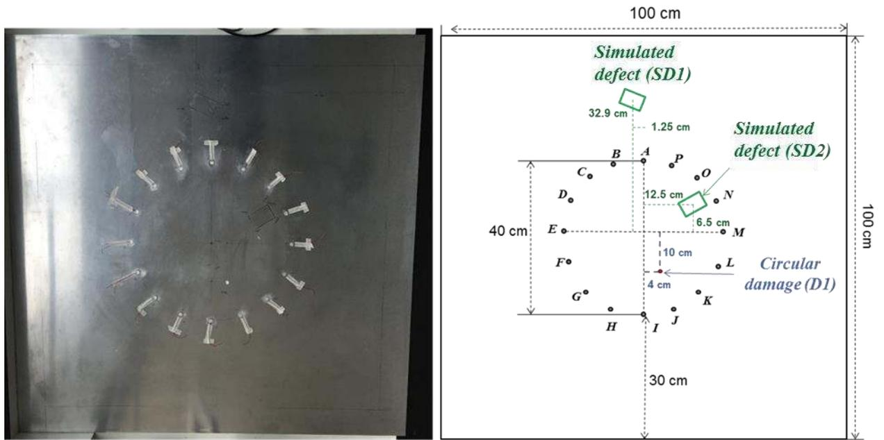
Figure 1: Picture (left) and schematic (right) of the aluminium plate (of dimension  $1\text{m} \times 1\text{m} \times 0.002\text{m}$ ) showing the position of the sensors (10 mm diameter and 0.5 mm thick), the location where the simulated defects were generated (by coupling effect) and the position where the real damage (circular hole of 10mm diameter) was inserted.
