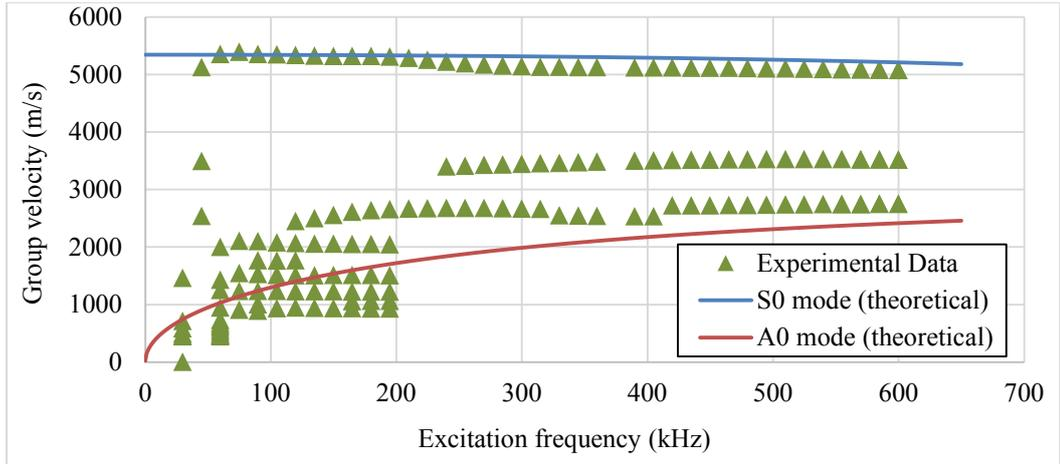
Figure 2: Dispersion curves of the aluminium plate.
