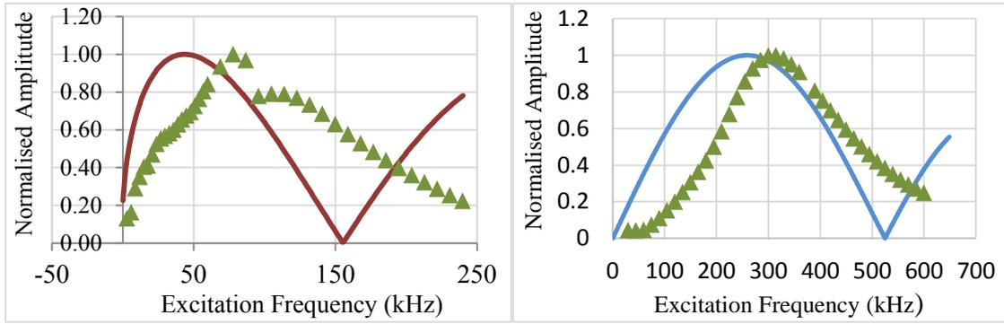
Figure 3: Tuning curve of the antisymmetric mode in red (left) and the symmetric mode in blue (right); the theoretical data (represented in green).
