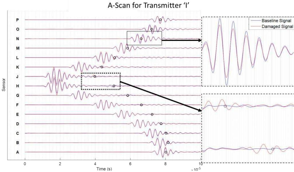
Figure 10: A-scans results obtained for the baseline signal, and after the implementation of a 10mm circular hole, when transducer 'I' is transmitting.
