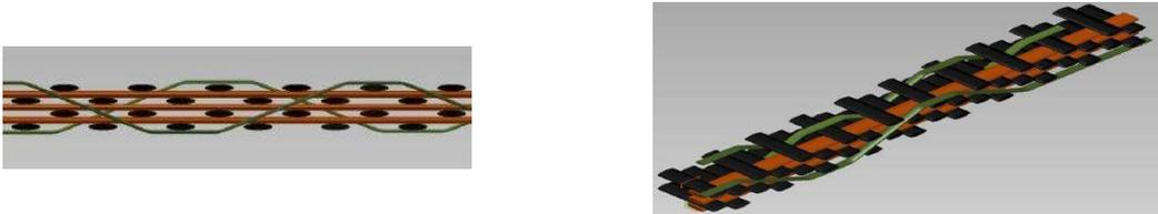
Figure 2: 3D Angle Interlock Woven Composite (through thickness and planar view) (orange: weft; black: warp; green: binder yarn) (Binder yarn goes all the way through-the-thickness and then returns back).
