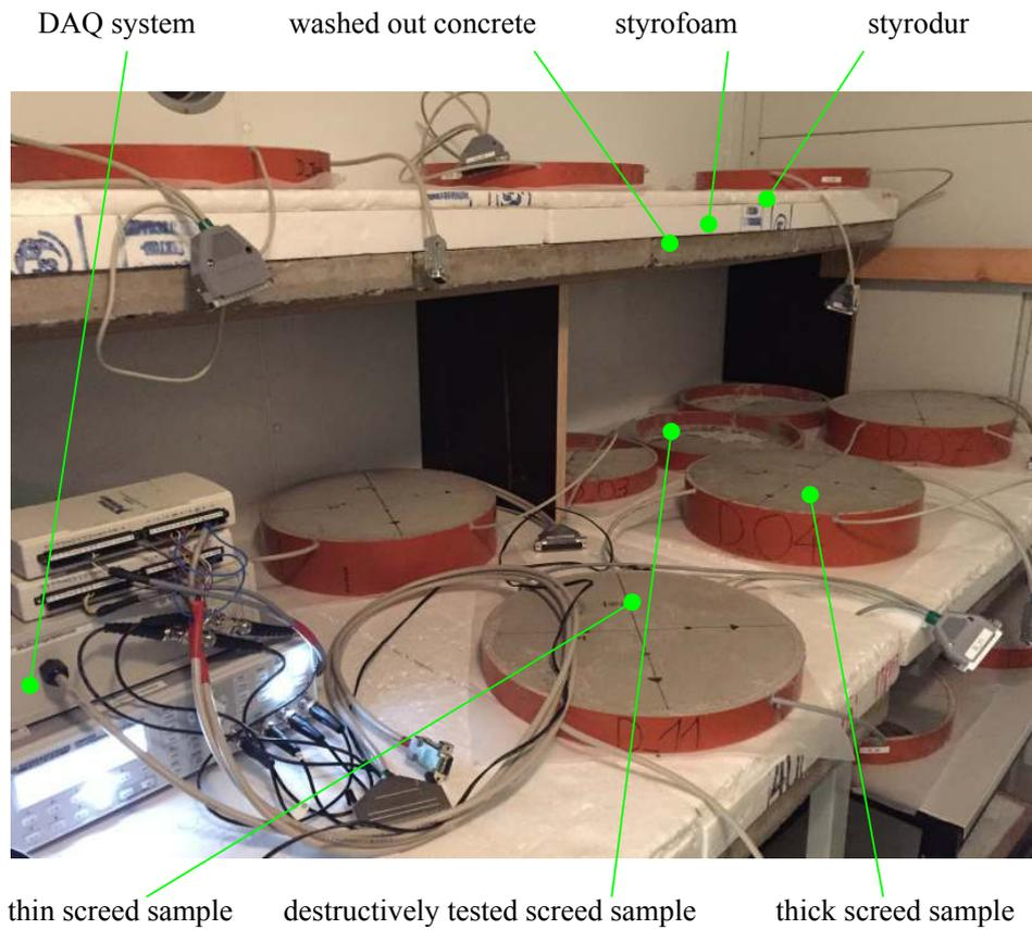
Figure 1: Screed sample storage in the ventilated climate chamber at 50% rH and 23° C
