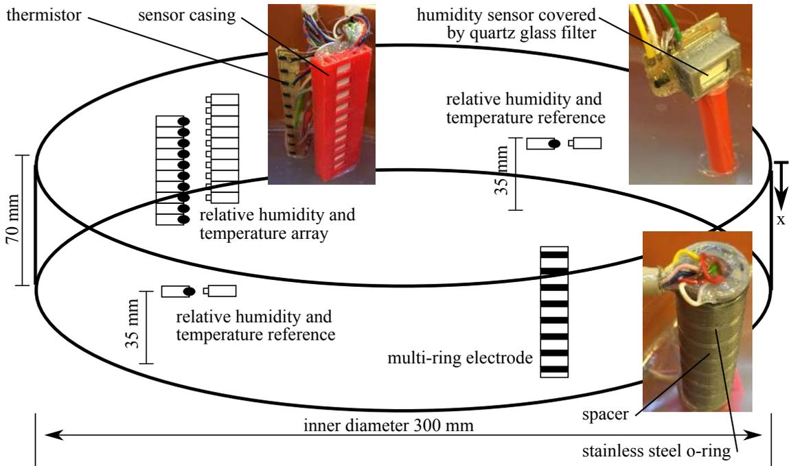
Figure 2: Sketch of the positions of the embedded sensors in the screed sample and photographs of the installed sensors before concreting; the x-coordinate is orientated from the top surface towards the bottom
