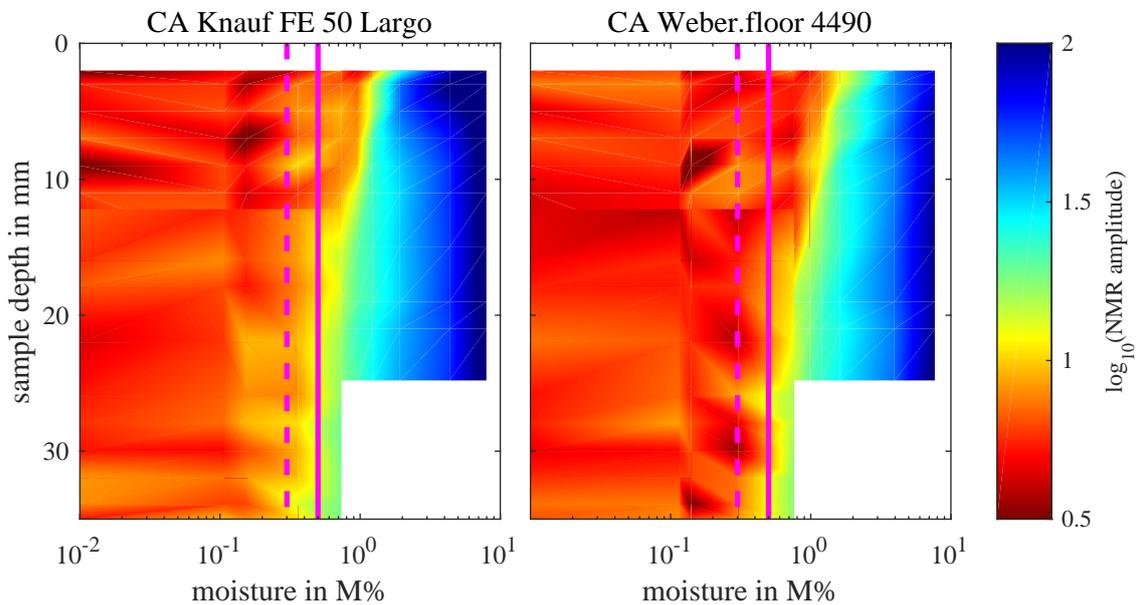
Figure 7: Logarithmic NMR amplitude over moisture (logarithmically scaled) including the flooring limits
