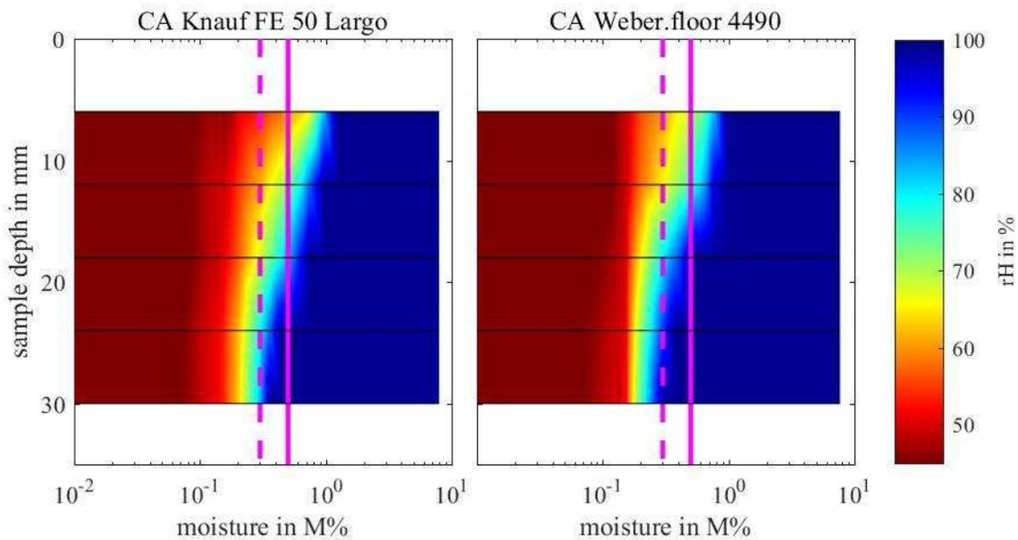
Figure 6: Evolution of the measured rH in % over moisture (logarithmic scaled); solid vertical magenta line: 0.5 M% limit for flooring; dashed vertical magenta line: 0.3 M% limit for flooring on heated screed
