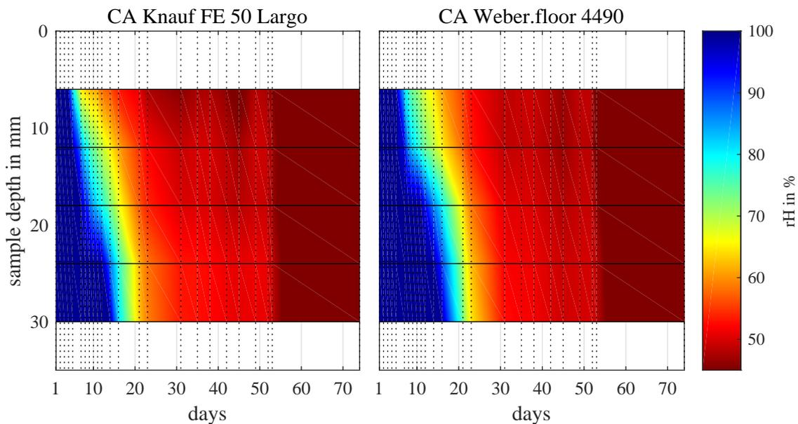
Figure 5: Measured rH in % across sample height and over time; the black horizontal lines mark the five measurement positions of the embedded sensors
