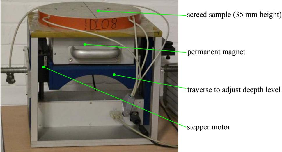
Figure 3: Photograph of the NMR-MOUSE with a thin screed sample measured from the bottom side
