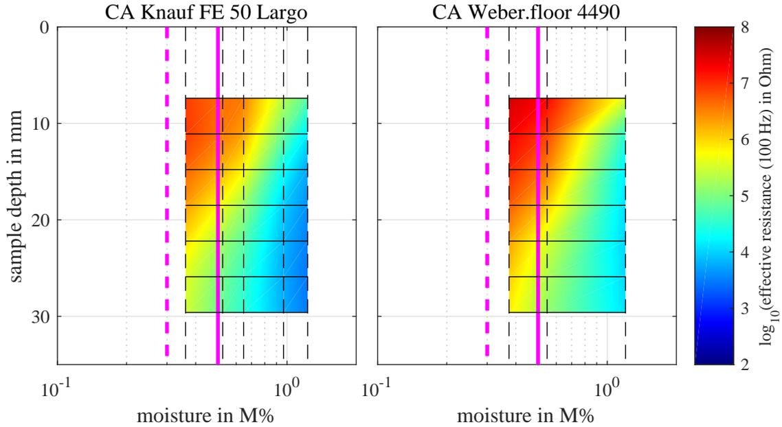
Figure 8: Logarithmic electric effective resistance of the MRE at 100 Hz AC versus moisture content (logarithmically scaled) including the flooring limits
