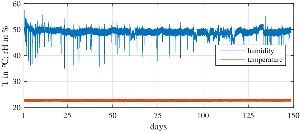
Figure 4: Temporal progress of the ambient humidity (blue line) and temperature (red line) in the climatic chamber
