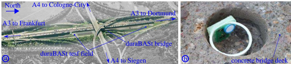
Figure 2: a) Depiction of the planned duraBAST test field including the duraBAST test bridge at the highway intersection “Köln-Ost”; b) Photograph of one RFID based humidity sensor before concreting in the duraBAST test bridge
