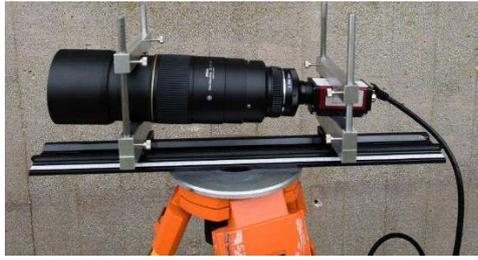
Figure 1: Mounting configuration of the camera and NIKKOR 300mm lens.
