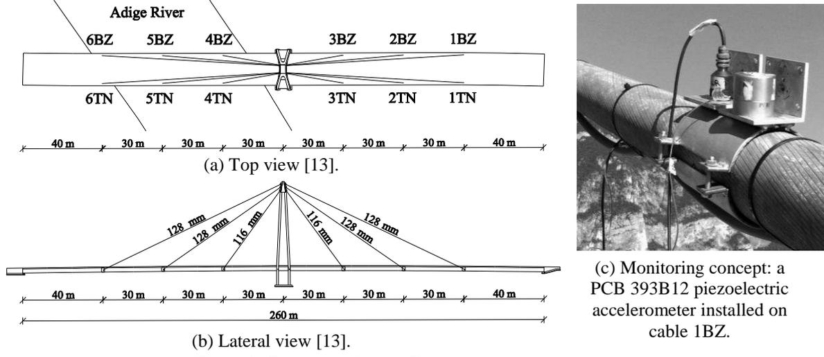
Figure 1: Geometry of Adige Bridge and monitoring concept.
