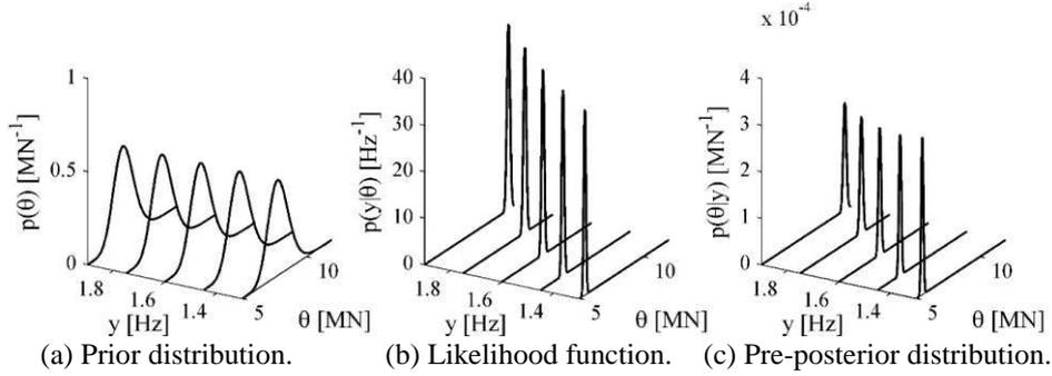
Figure 2: Distributions involved in the prediction of the uncertainty that affects the tension force of stay cable 1BZ.
