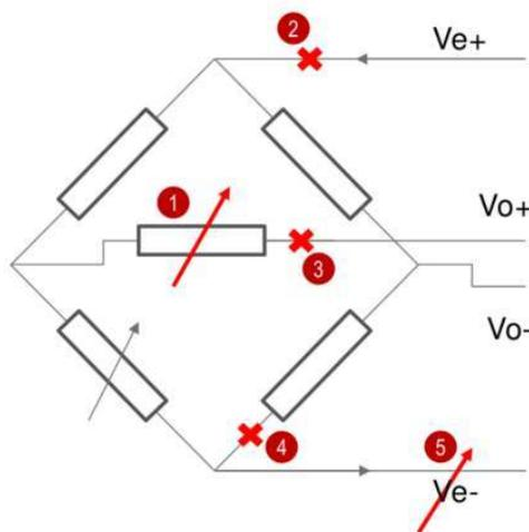
Figure 3 : Wheatstone Bridge sensor labelled with the five fault types  $\{F1, F2, F3, F4, F5\}$
