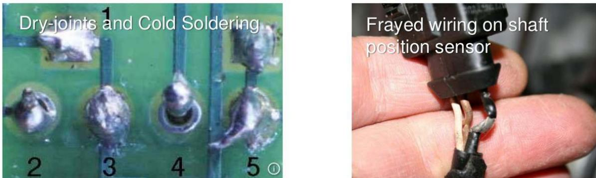
Figure 1 : Example sensor with catastrophic failures
