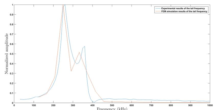
Spectrum of the tail. Comparison of FEM and experimentally results for PMMA
