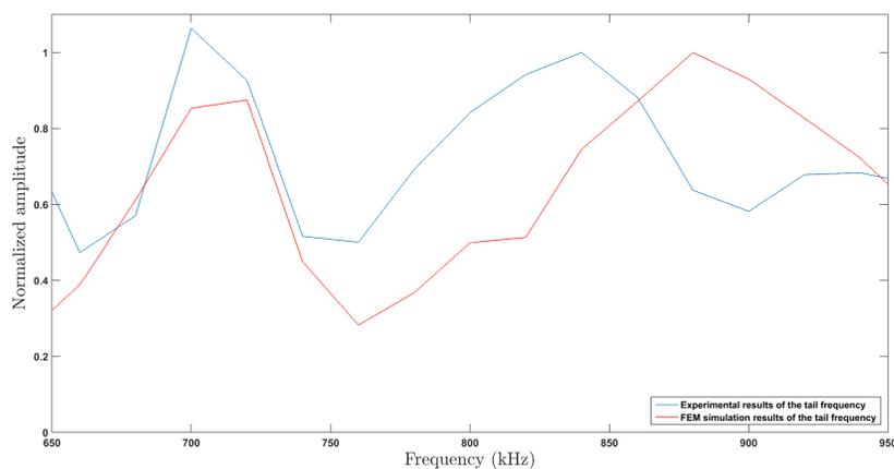
Spectrum of the tail. Comparison of FEM and experimentally results for aluminium
