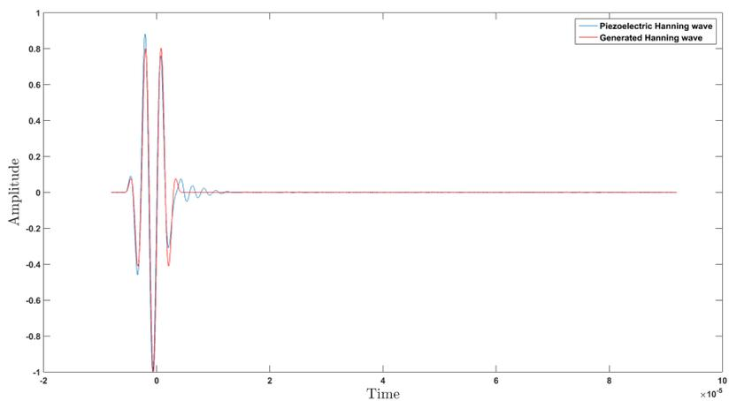
Comparison between generated wave and experimentally measured in PWAS receiver for aluminium
