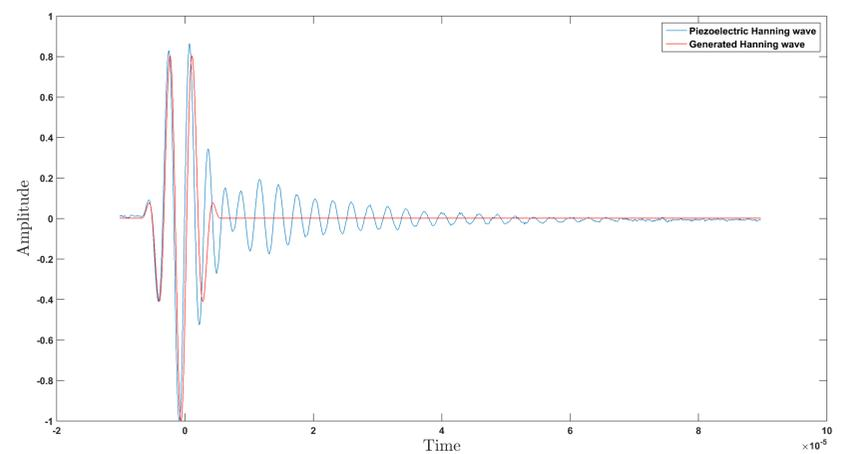
Comparison between generated wave and experimentally measured in PWAS receiver for PMMA
