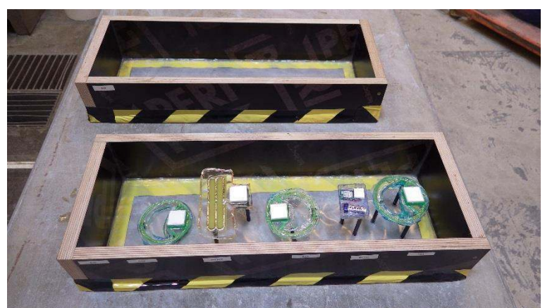
Test specimen with RFID systems before filling with concrete
