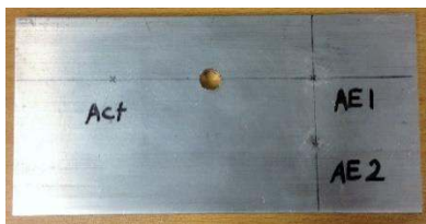
a. Plate (152x76x6.3 mm) b. Block 1 (152x50.8x25.4 mm) c. Block 2 (152x50.8x38.1 mm)
