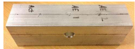
a. Plate (152x76x6.3 mm) b. Block 1 (152x50.8x25.4 mm) c. Block 2 (152x50.8x38.1 mm)
