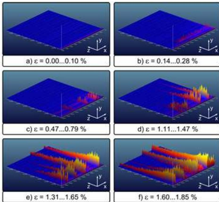
Figure 7. Process topography of HFIM for different strain conditions (a–f)
