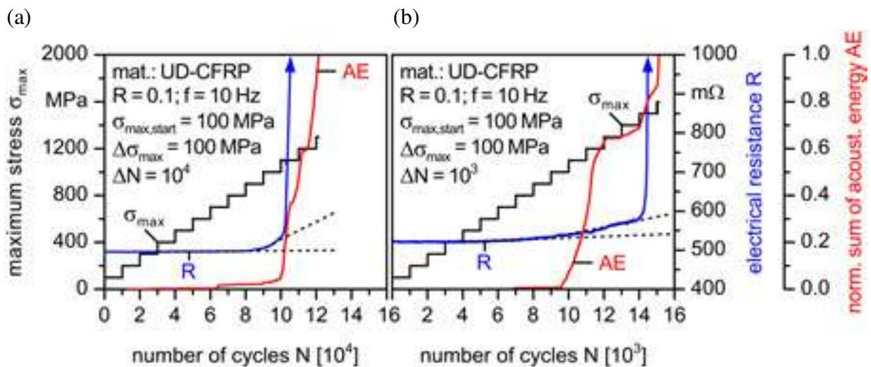
Figure 8. Multiple step tests with step length (a)  $10^4$  and (b)  $10^3$  load cycles
