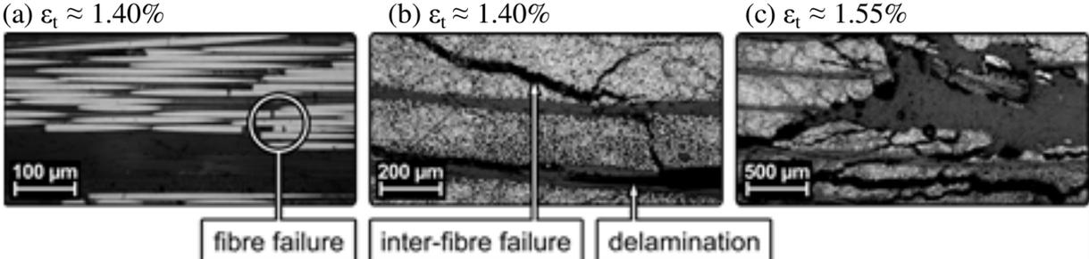
Figure 4. Light micrographs for different strain conditions (a-c)
