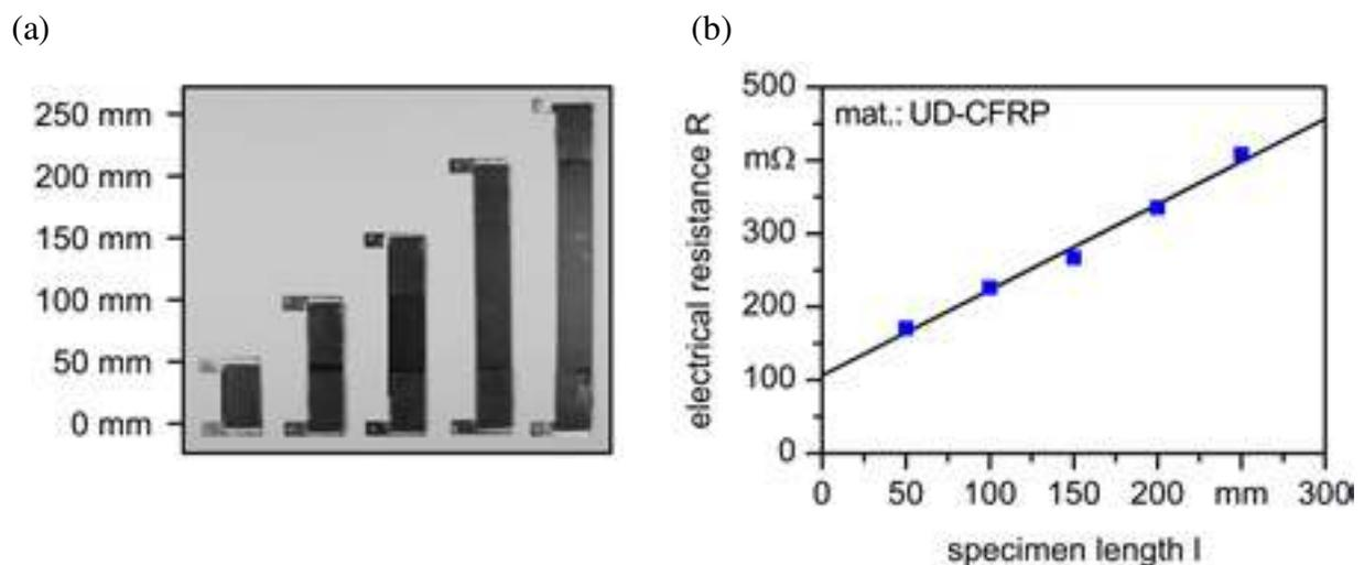
Figure 1. (a) Test specimens and (b) graph to determine the conductor resistance
