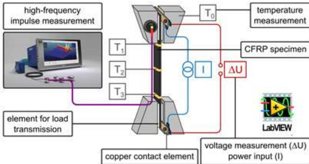
Figure 2. Experimental setup for quasi-static and cyclic tests (schematic)
