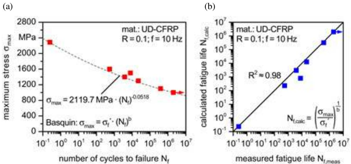
Figure 9. (a) Woehler curve as function of maximum stress versus number of cycles to failure, (b) Correlation between measured and calculated life time according to Basquin equation
