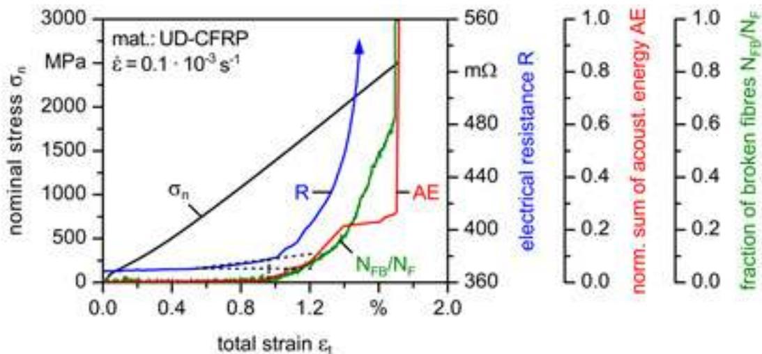
Figure 3. Quasi-static tensile test at  $\dot{\epsilon} = 0.1 \cdot 10^{-3} \text{ s}^{-1}$
