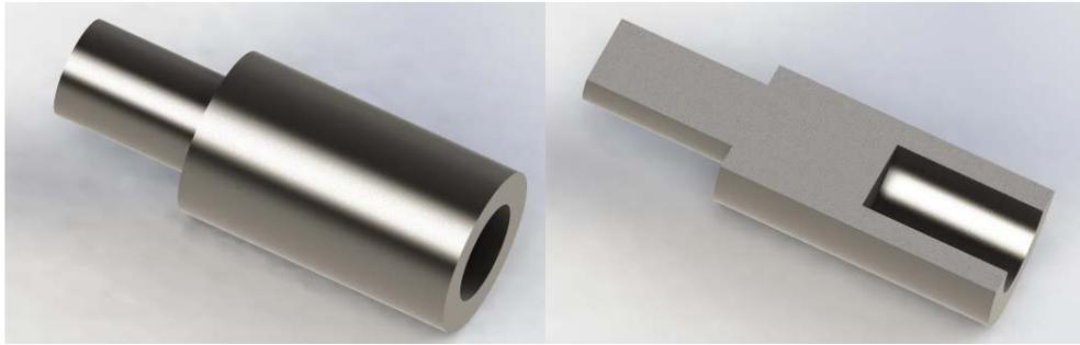
Figure 1: Dimensional and surface determination scaling artefact
