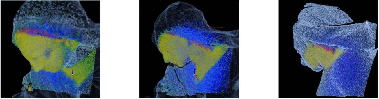
Figure 7: XRF images from all three angles mapped onto tomographic reconstruction. Colors represent energy the same energy windows as utilized for Fig. 5.
