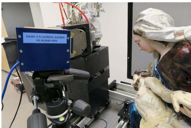
Figure 2. The Pieta installed on the rotational table in the CT/XRF setup.
