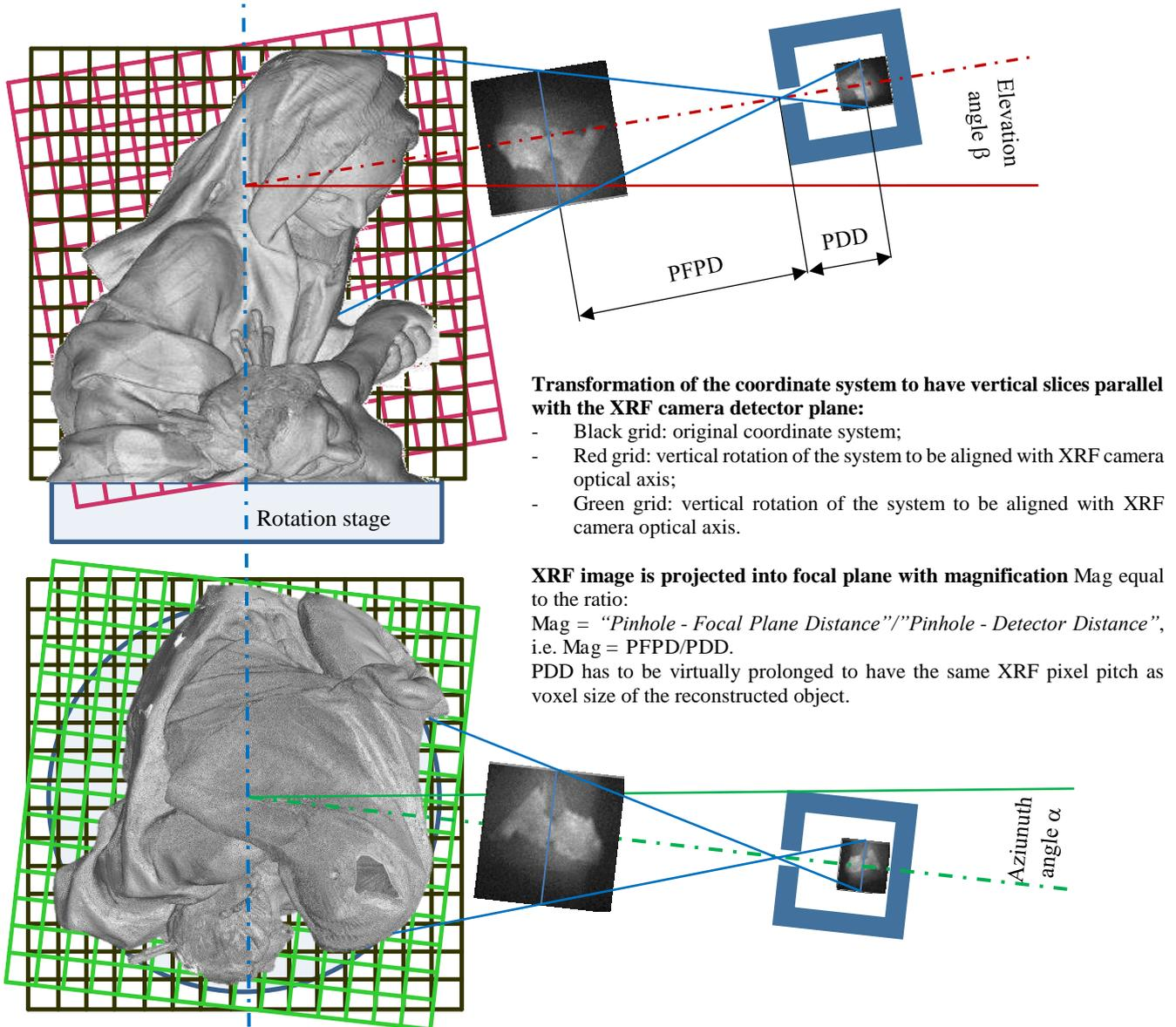
Figure 3. The principle of the XRF imaging and mapping.
