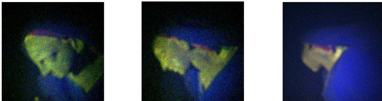
Figure 5. XRF image in the RGB representation. Left one was taken with azimuth angle  $84^\circ$ , middle image with azimuth  $54^\circ$  and right one with azimuth  $24^\circ$  respectively. The mixture of materials is expressed by the resultant color: R 3-7 keV (covering iron XRF peak), G 8-16keV (zinc), B 18-28keV (silver and scattered photons).
