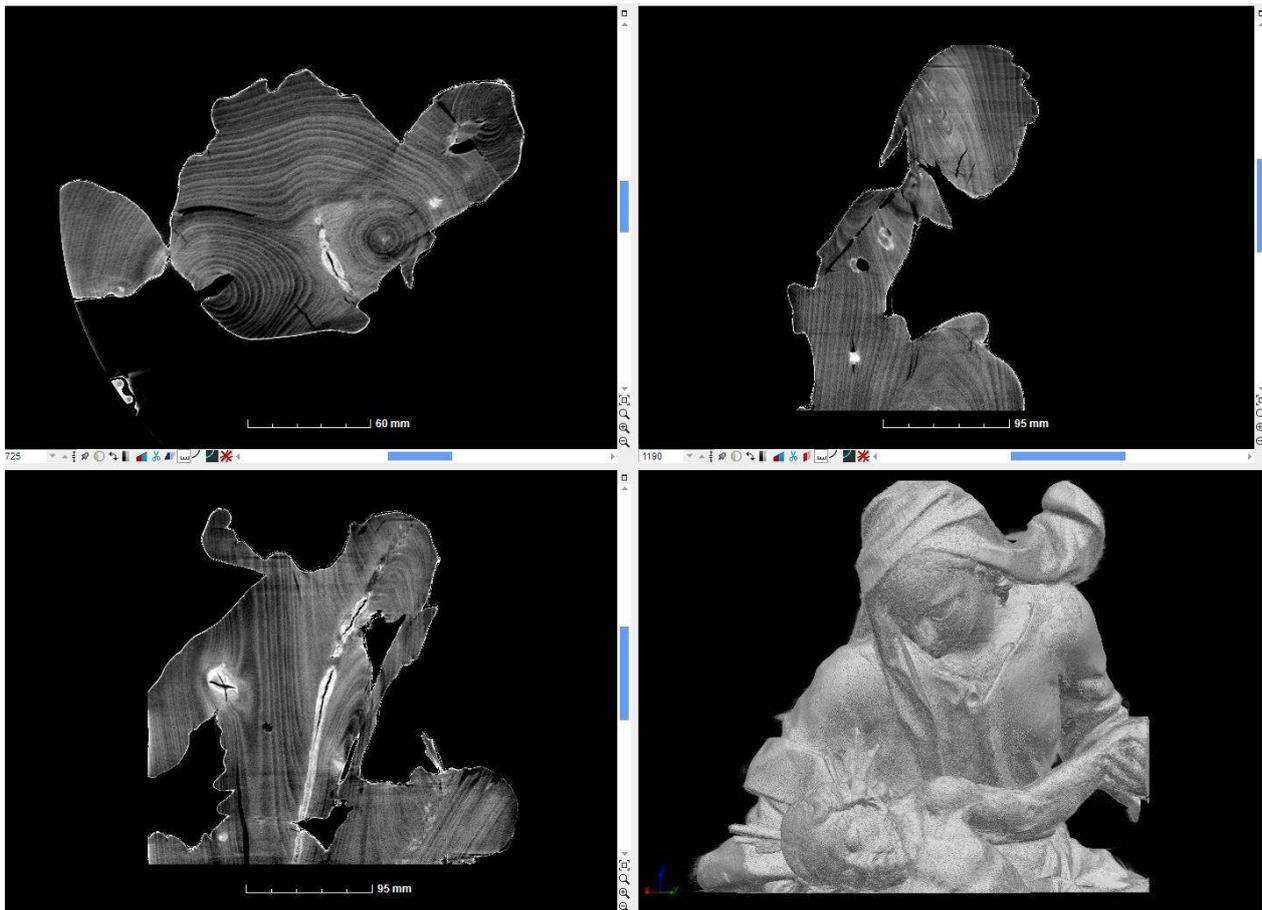
Figure 4: Visualization of the reconstructed Pieta. Wooden structure is well visible. Polychrome layer covering sculpture, which has a higher density than wood, is manifested as white-black contour surrounding crossections.
