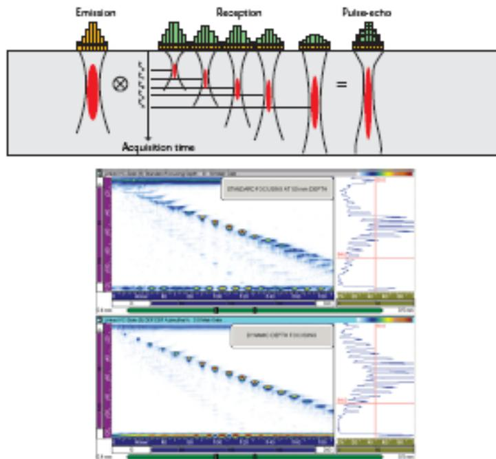
**Figure 3-33** Dynamic depth focusing (DDF): (a) principle—resulting beam by convolution; (b) comparison between standard phased array focusing and DDF on the depth-of-field. Note the detection of two SDH in the near-surface zone by DDF and missed by standard phased array focusing.
