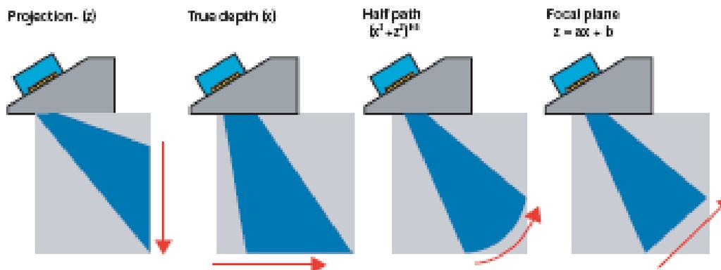
Figure 3-26 Type of focusing for linear phased array probe.
