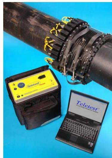
In addition, collar sizes of 4-24" provide the user with the ability of testing 4-48" pipe sizes by simply linking the collars together.
