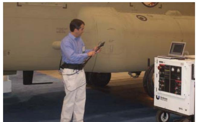
*iGPS receivers incorporated into probe stay within reach of the transmitters surrounding the aircraft.*
