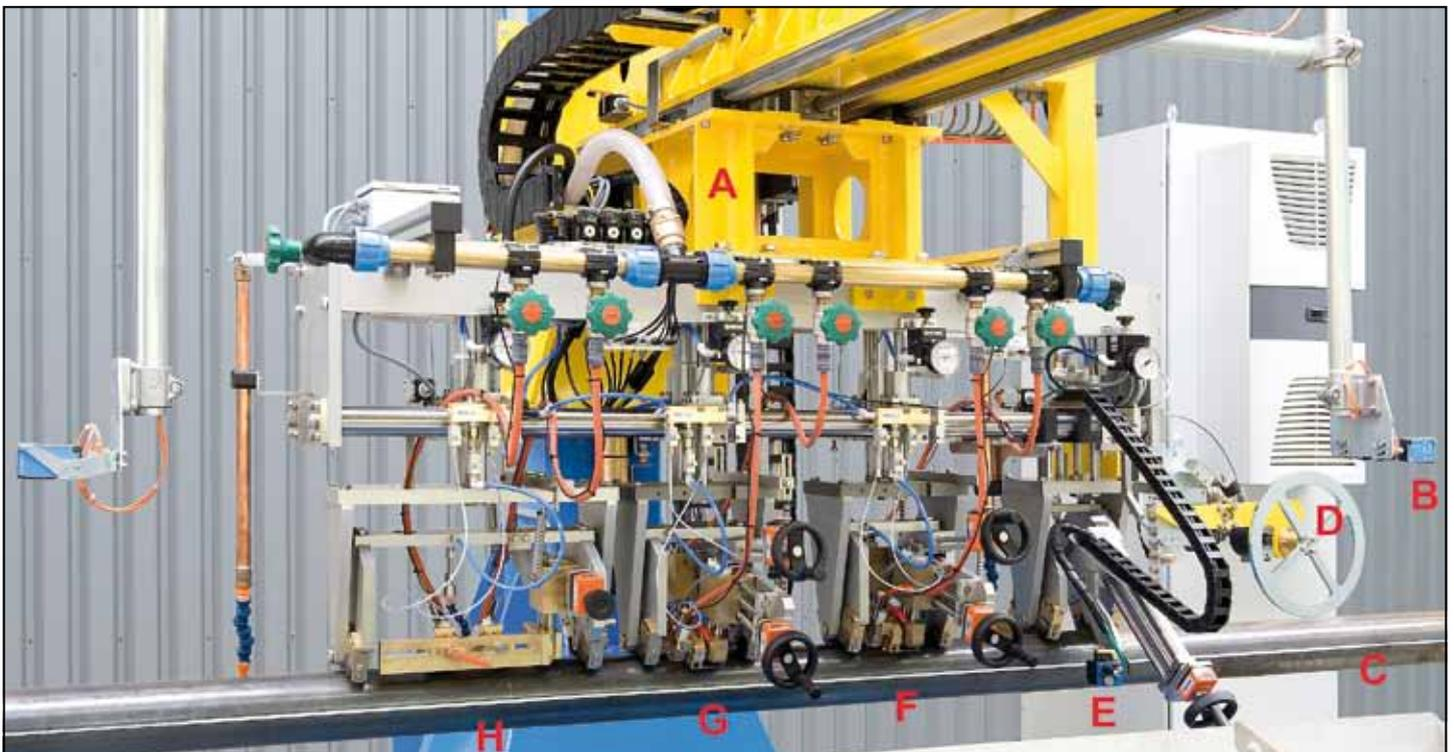
**ECHOGRAPH-SNHF Testing system for welded pipes** A: machine frame B: light barrier on entry side C: pilot line D: position encoder wheel E: camera for seam tracking F: pair of probes for internal longitudinal defects G: pair of probes for external longitudinal defects H: pair of on-bead probes for transverse defects
