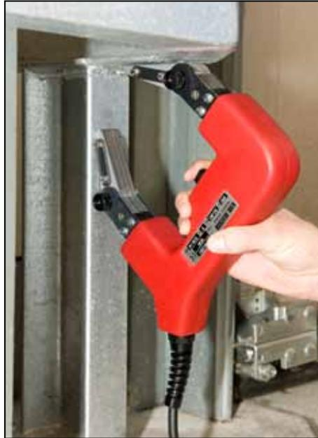
DEUTROPULS hand yoke with flexible attachment poles
