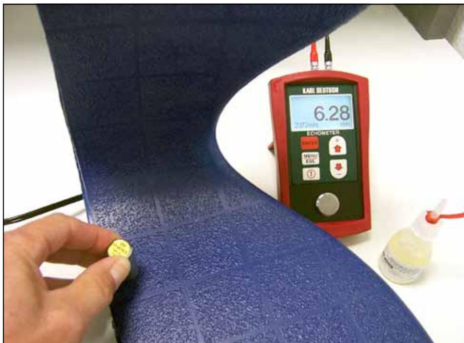
and for edges DSE 4.2/4 PB 8). To test the inside radius, in this case the area between seat and backrest, a proper coupling of the probe must be checked in advance. Incorrect coupling of the probes can cause systematic errors while measuring. If the surface is extremely curved a measurement might not be possible at all. In our example, the curvature of the seats was large enough to enable proper mea-
