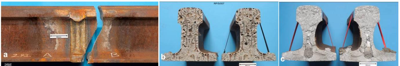
Figure 2 Defective samples; (a) failure; (b) porosity; (c) shrinkage.
