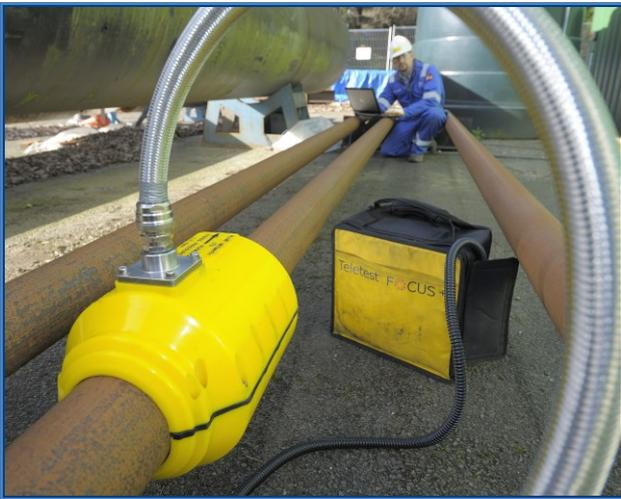
Figure 1: The 4 inch Teletest Permamount system
