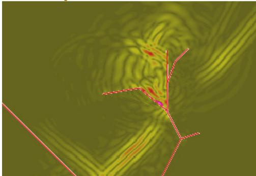
The CIVA ATHENA2D module allows to store beam snapshots that can be used to generate and visualize a video of the of the beam/flaw scattering. Such a video might be very interesting to visualize the physical phenomena that are created when the field interacts with flaws and/or specimen boundaries. To generate a video of the field propagation and interaction with the flaws and/ or specimen boundaries the steps are the following: [Read more and visualize a presentation video](#).
