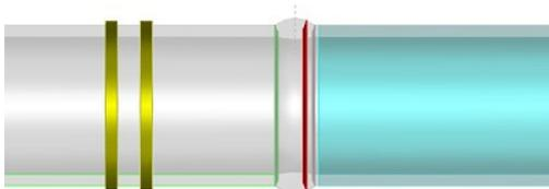
A new CIVA GWT version is going to be released in the next weeks. New capabilities will be available. In particular CIVA 11 GWT will predict the response of a 2D geometrical discontinuity of the waveguide. It may be for example an axisymmetric weld, groove or section transition between pipes of different diameters. Moreover a flaw may be inserted close to the discontinuity, CIVA will then handle the prediction of the echoes from the flaw and from the discontinuity.
