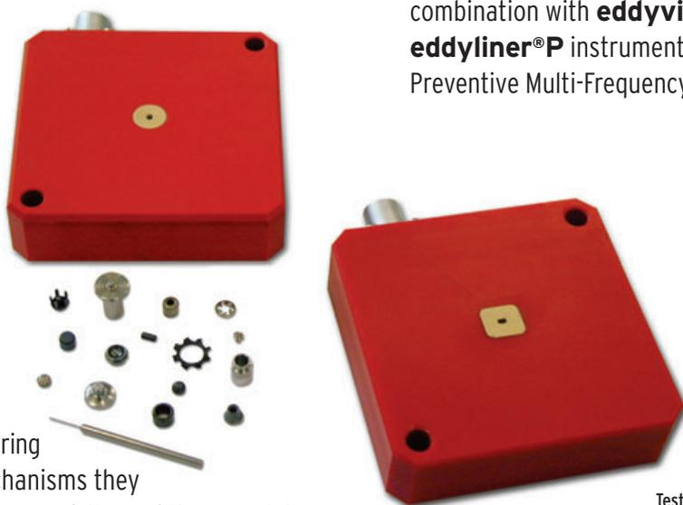
Test coils with very small parts
