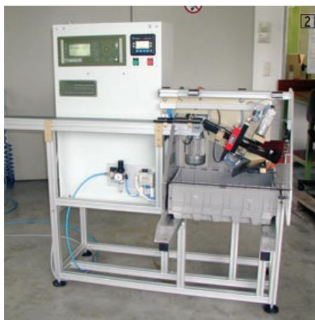
Photo 2: Semi-automatic test system for stampings
