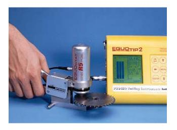
The EQUOSTAT hardness tester is a light weight, yet powerful portable hardness tester for all metallic materials.
